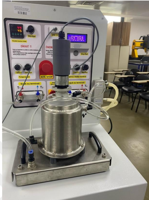
Figure 3.1. The jacketed stirred heat exchanger used in the experimental study
