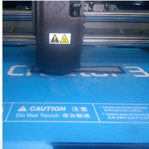
Figure 2.5. Production of tensile test sample on a FlashForge material extrusion device.
