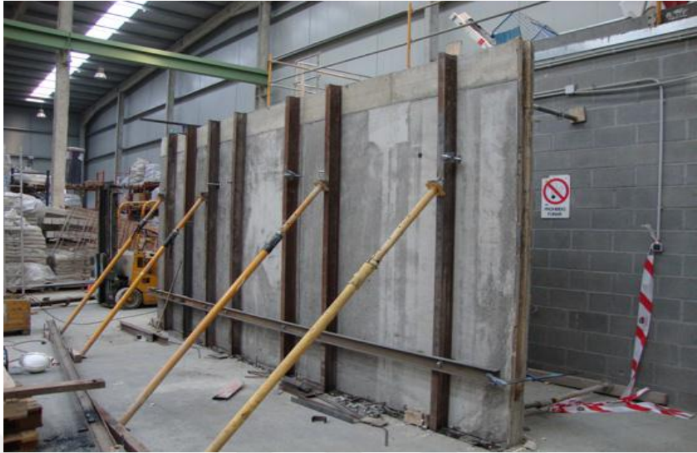
Figure 2.11 SFRSCC wall (Orbe et al., 2012)
