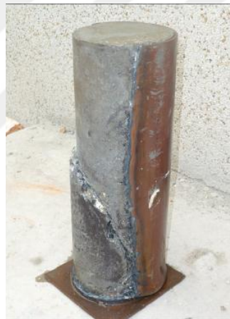
Figure 2.30 Shear failure plane in concrete core (Yi-yan et al., 2015)
