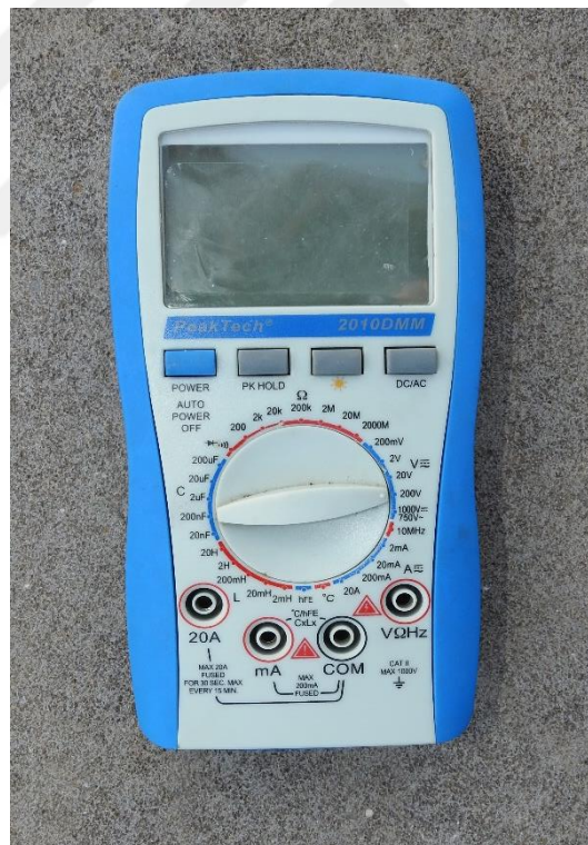
Figure 3.12 Multimeter devices (a) for measuring electrical current and (b) for measuring the voltage.
