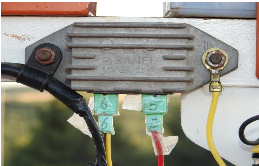
Figure 3.7 The voltage regulator.
