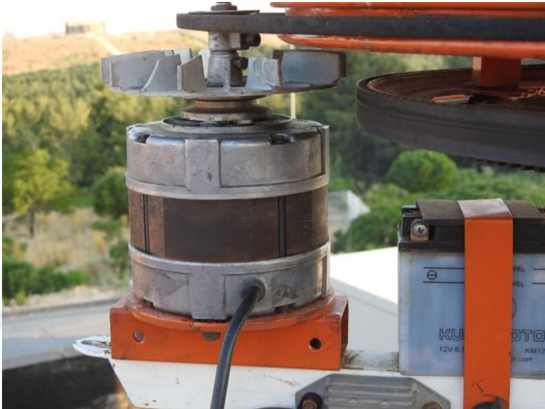
Figure 3.5 Permanent magnetic generator.
