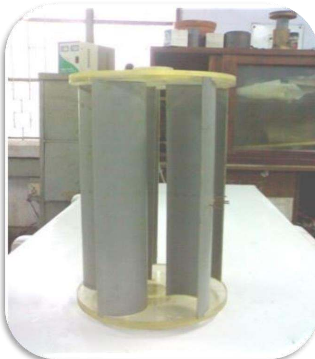
Figure 2.9 Five bladed vertical axis vane type rotor [31].
