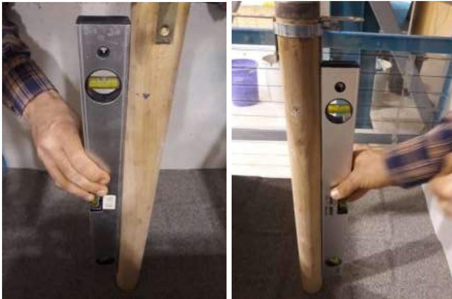
Figure 4.10. Checking vertically of the model pile
