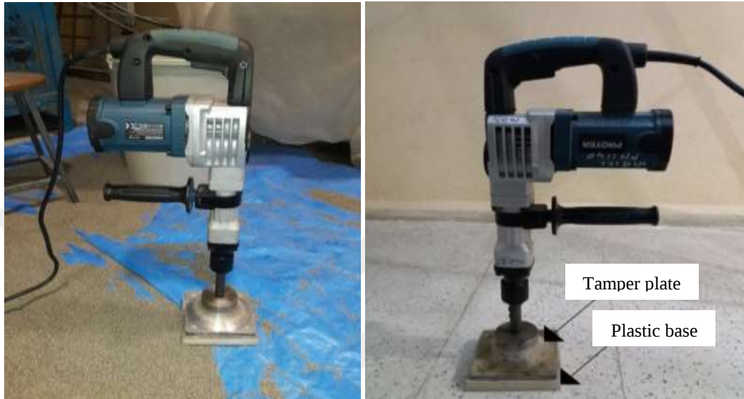
Figure 4.4. Proter brand electro-pneumatic hammer
