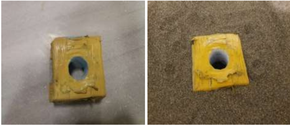
Figure 4.18. Styrofoam prepared for the model pile shaft friction test
