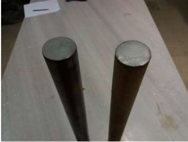
Figure 4.9. Galvanized steel plate at the bottom of the model piles
