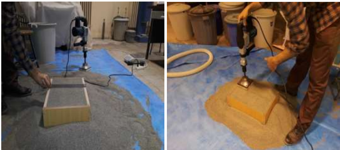
Figure 4.5. Calibration of relative densities in the laboratory
