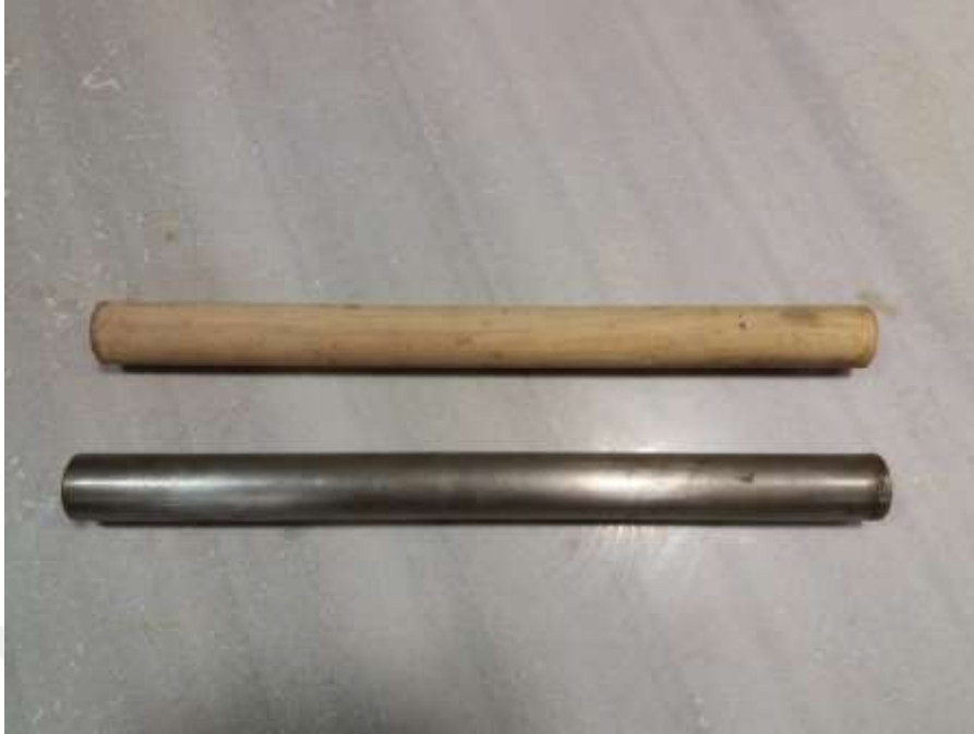
Figure 4.2. Timber and steel model piles
