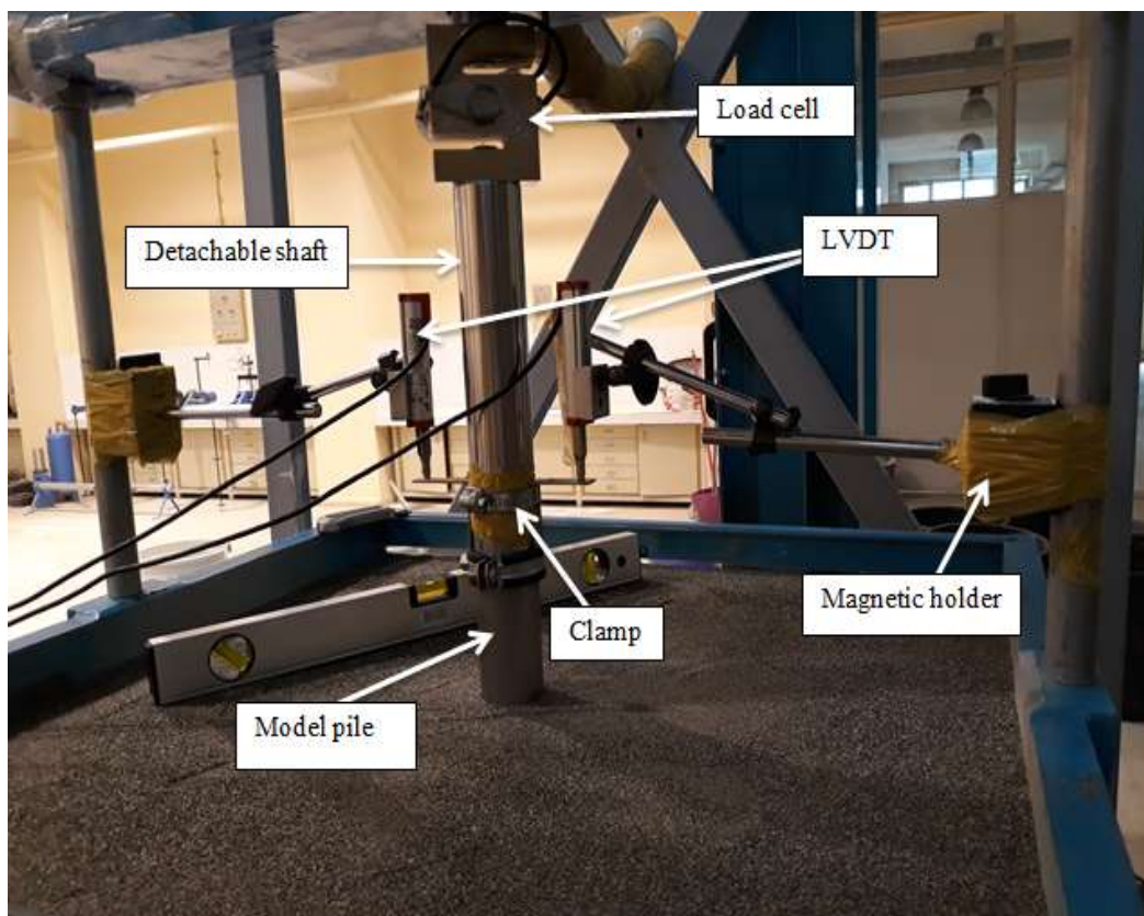
Figure 4.11. Installing LVDT on model pile.
