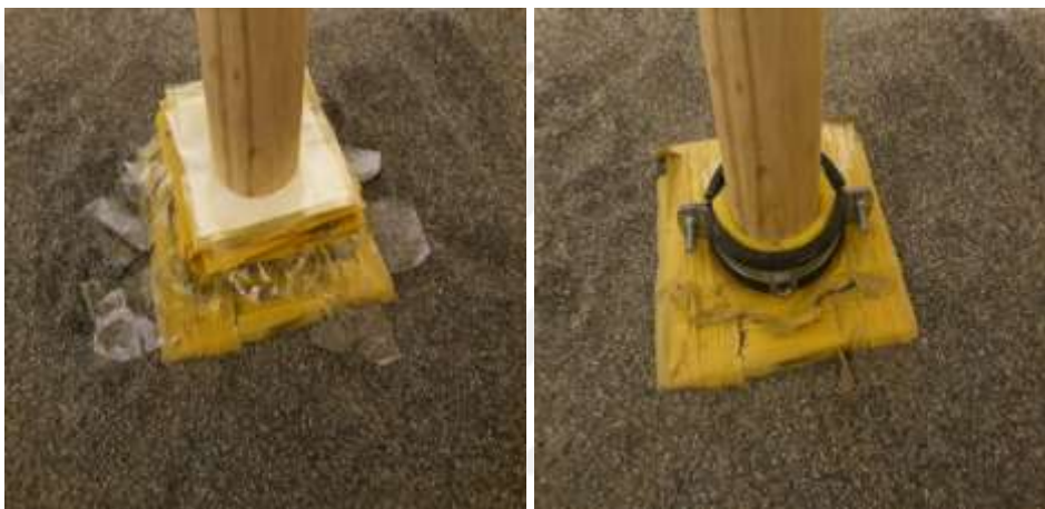
Figure 4.19. Timber model pile Prepared for a shaft friction resistance test.
