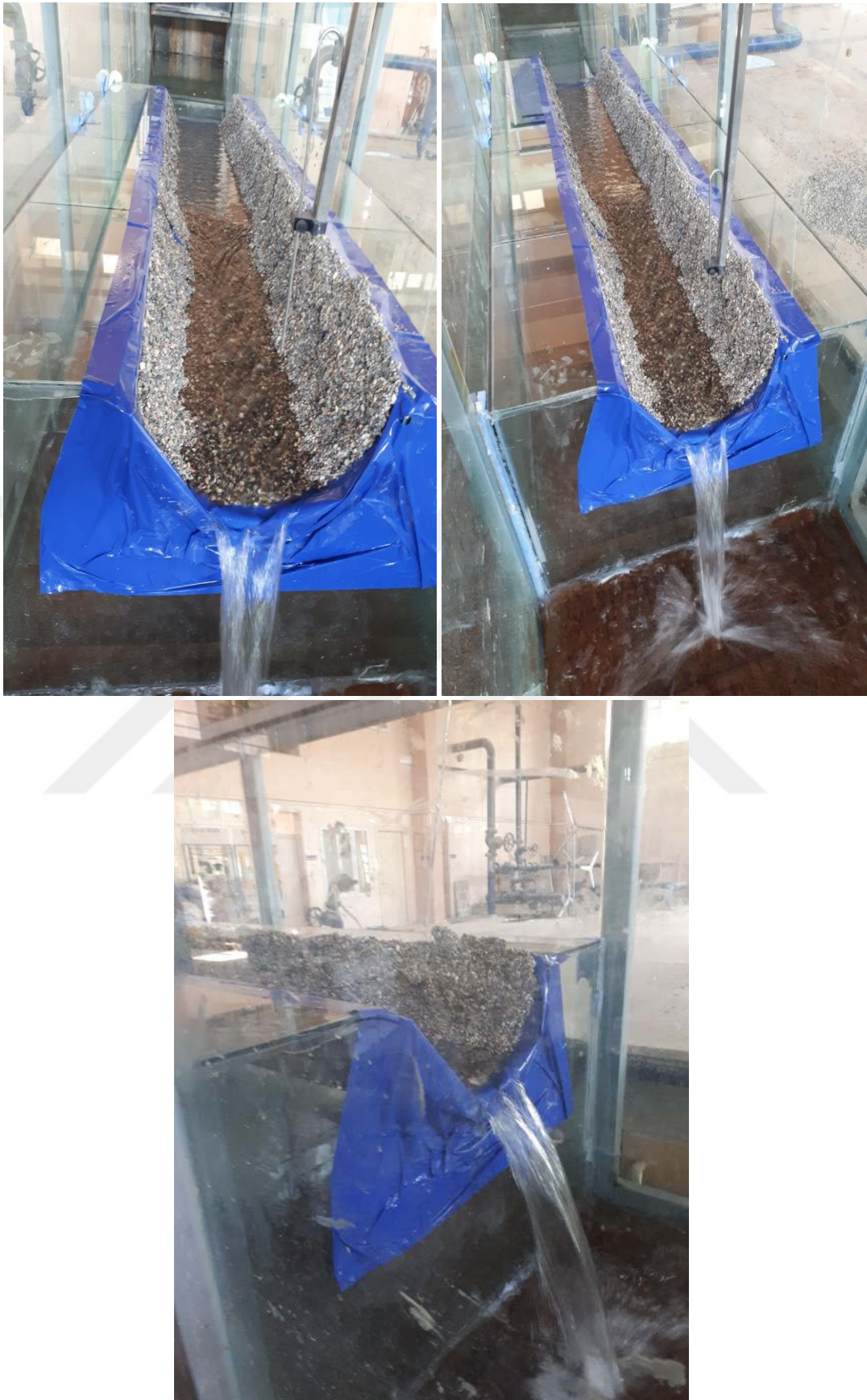
Figure 4.11 Free Overfall in Semicircular Channels with (2 mm) Roughness on Bottom
