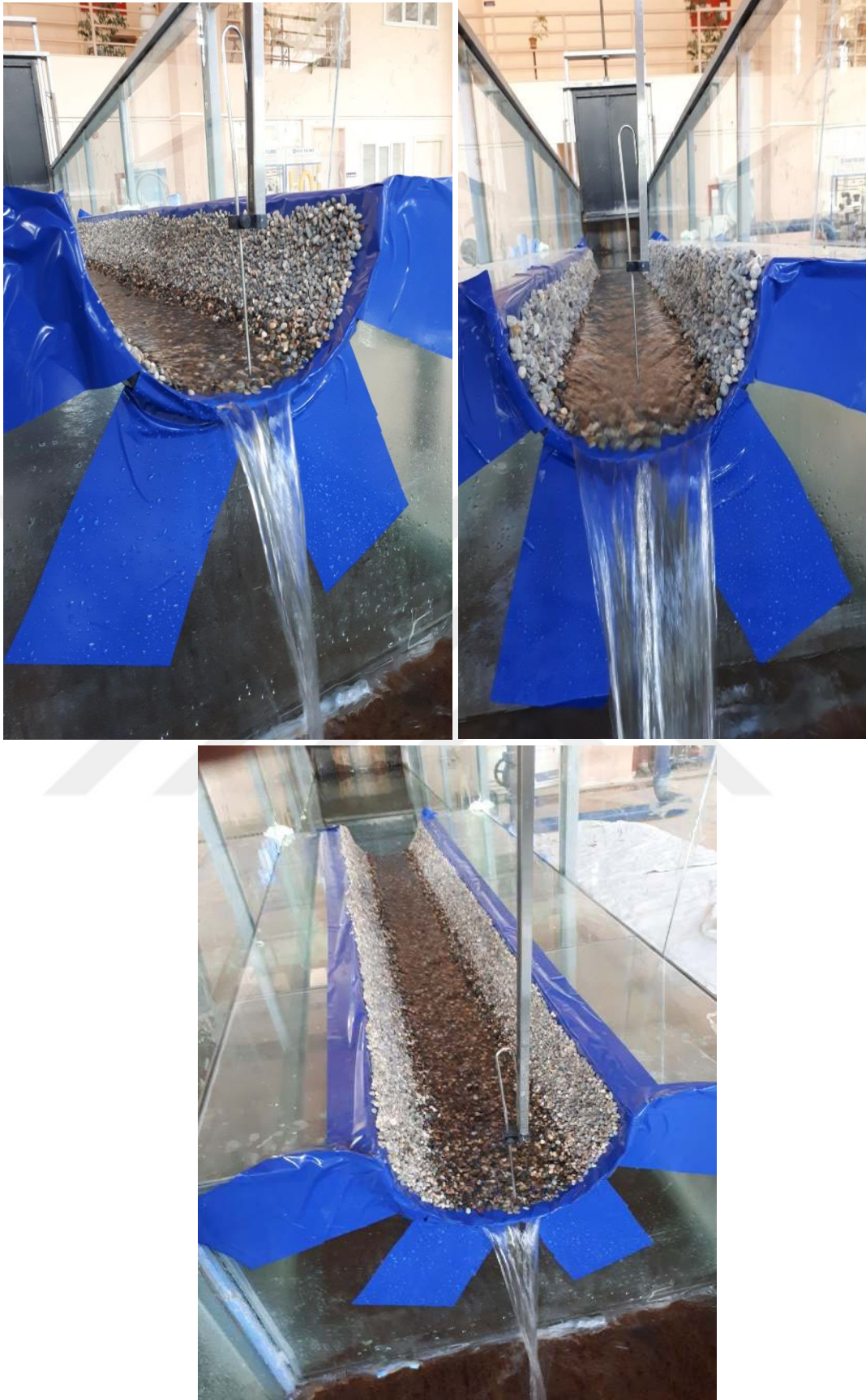
Figure 4.12 Free Overfall in Semicircular Channels with (4.75 mm) Roughness on Bottom
