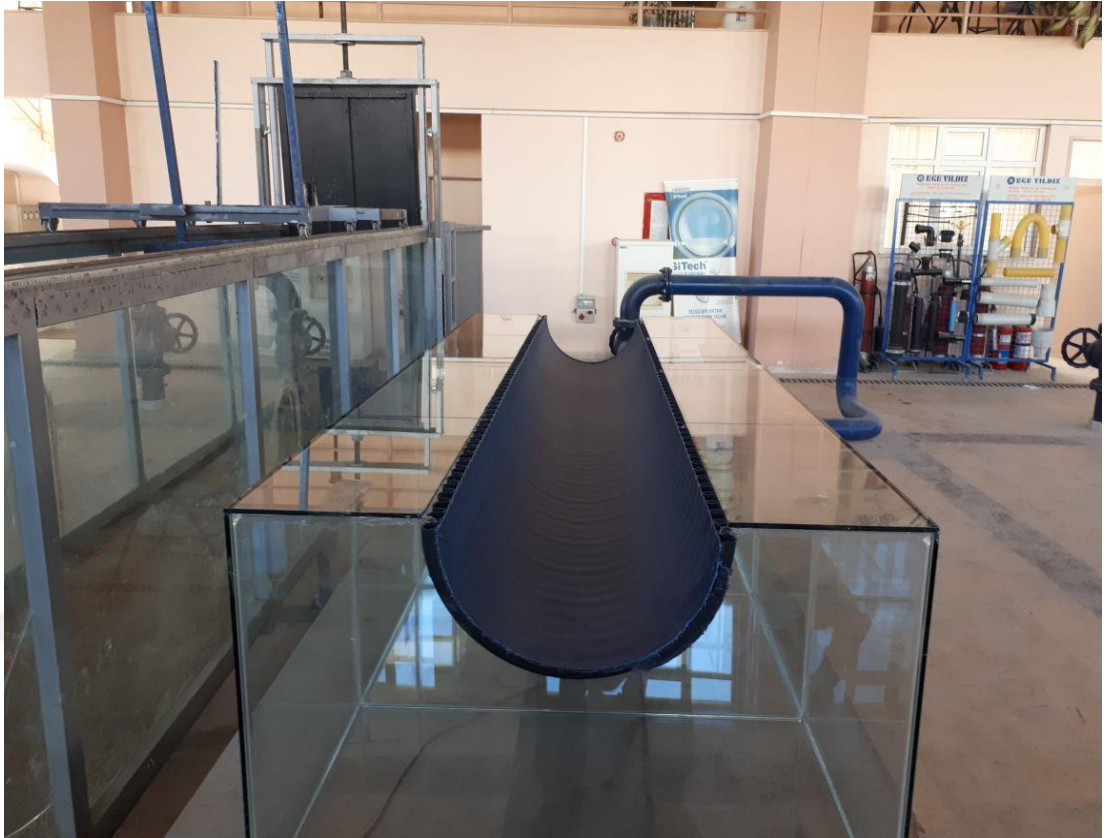
Figure 4.9 (c) Semicircular Channel (View 1)
