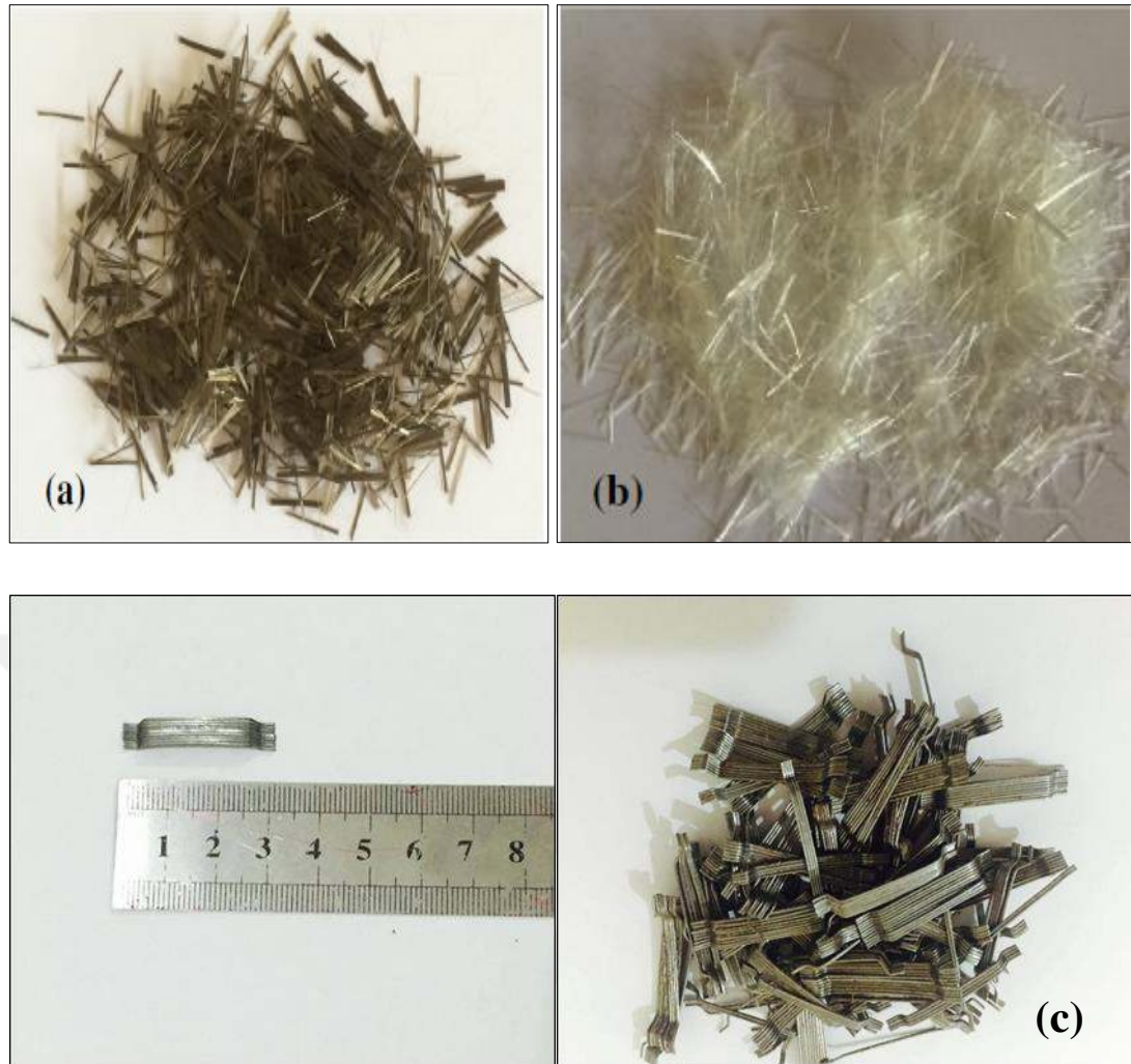
Figure 3.1 (a) basalt fibers, (b) glass fibers, and (c) steel fibers.
