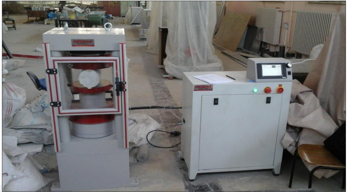
Figure 3.6 Splitting tensile test machine
