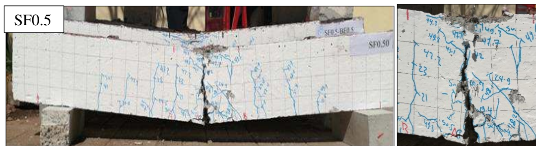
Crack pattern and failure mode for CB
