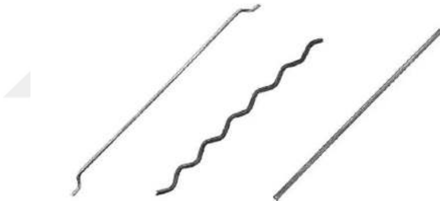
Figure 2.3 Fiber shapes (Ghoraishi et al., 2011)
