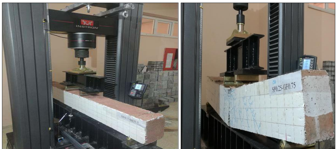
Figure 3.7 Flexural Beam test and beam failure
