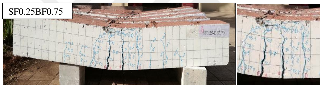
(a) Crack pattern and failure mode for group A
