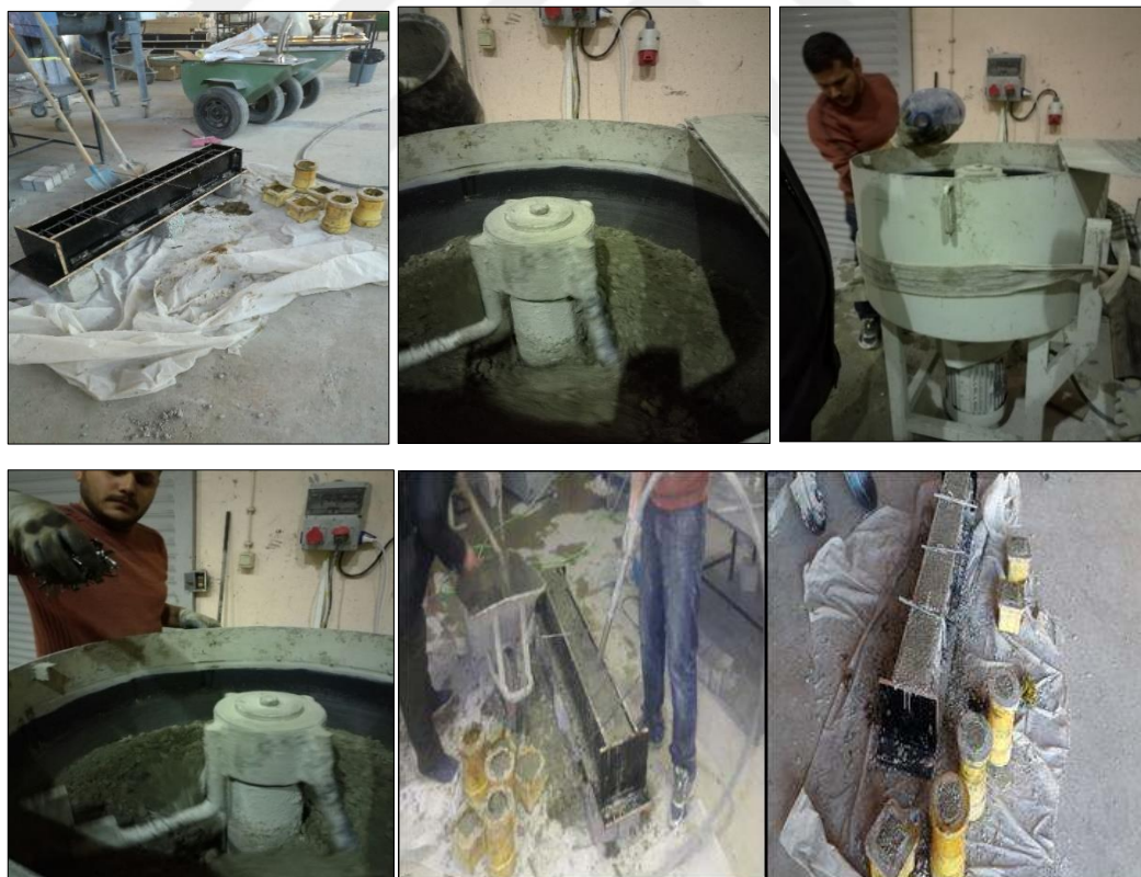
Figure 3.4 Proportioning, mixing and casting of beam specimens
