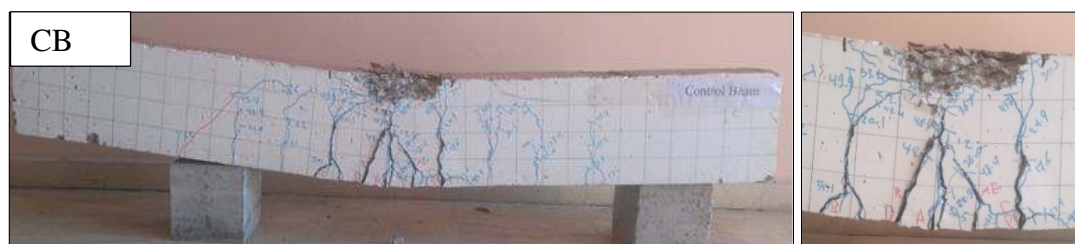
Crack pattern and failure mode for CB
