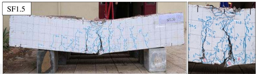
(a) Crack pattern and failure mode for group A
