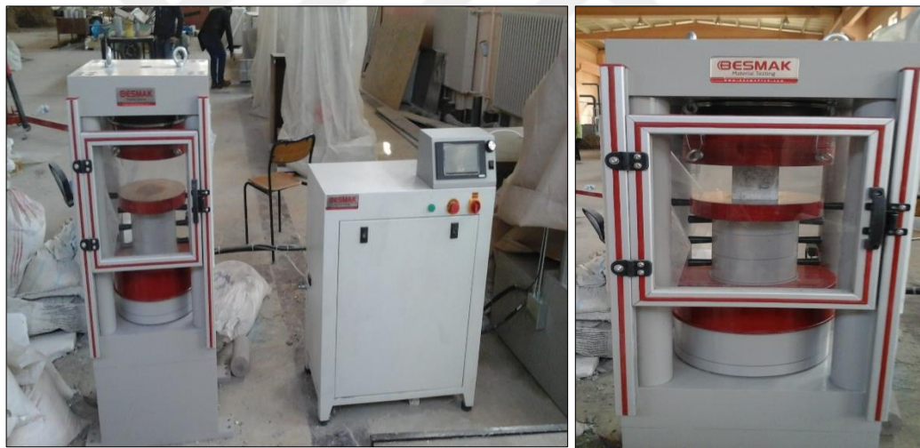
Figure 3.5 Concrete compressive test machine
