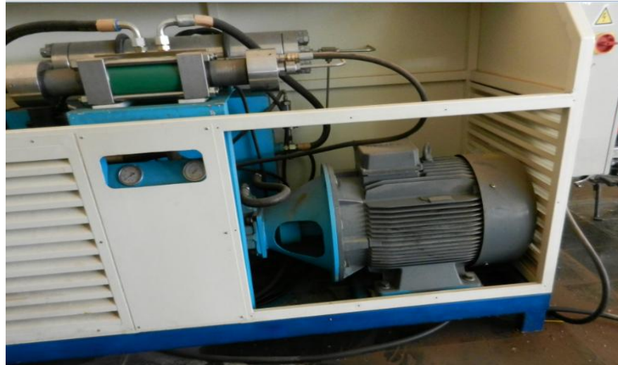
Figure 3.8 Abrasive water jet machine pumping system
