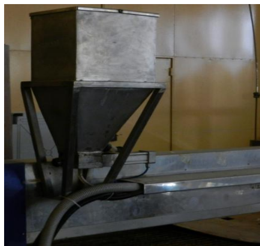
Figure 3.22Structure of abrasive material hopper
