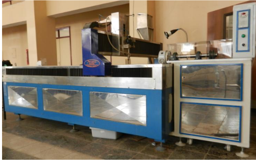
Figure 5.2 AWJ machine coupled with the turning system
