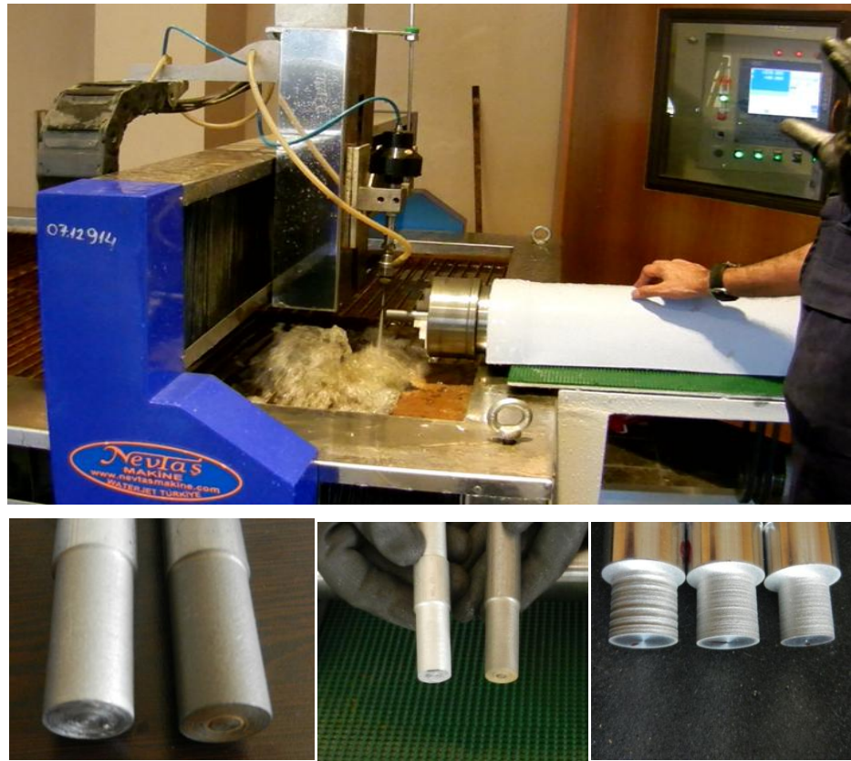
Figure 4.17 Operation of the turning system and products obtained
