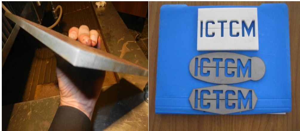
(a)Stainlesssteel cut by AWJ ( b)Carbon steel cut by AWJ
