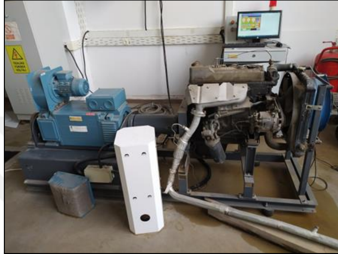
Figure 30. Mitsubishi Canter 4D31 diesel engine setup
