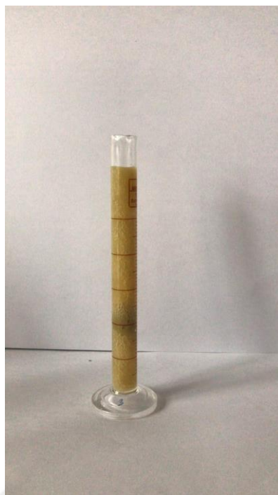
Figure 4.5 A picture of swelling capacity of okra mucilage on test tube
