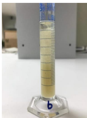
Figure 4.15 A picture of okra mucilage water emulsion after 24 hr of duration
