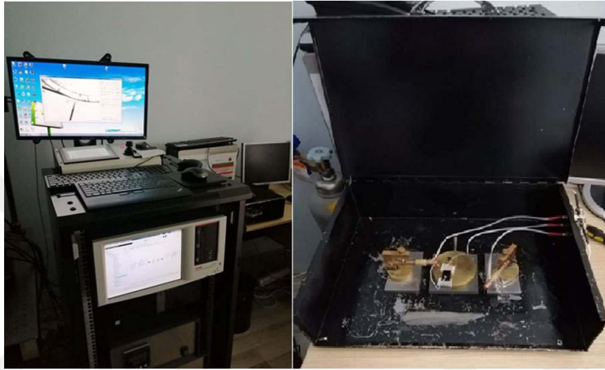
Picture 3.2. C-V measurement system at NURDAM.
