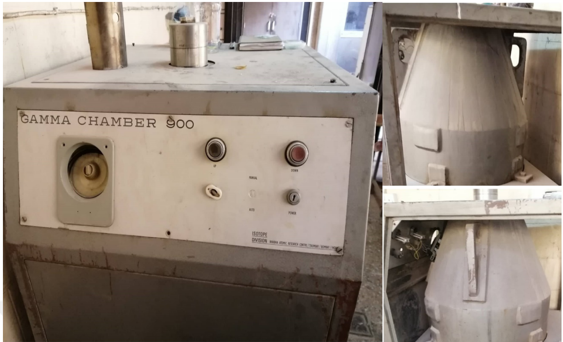
Picture 3.3. Irradiator chamber 900 Co-60 gamma-ray source system at the University of Baghdad.
