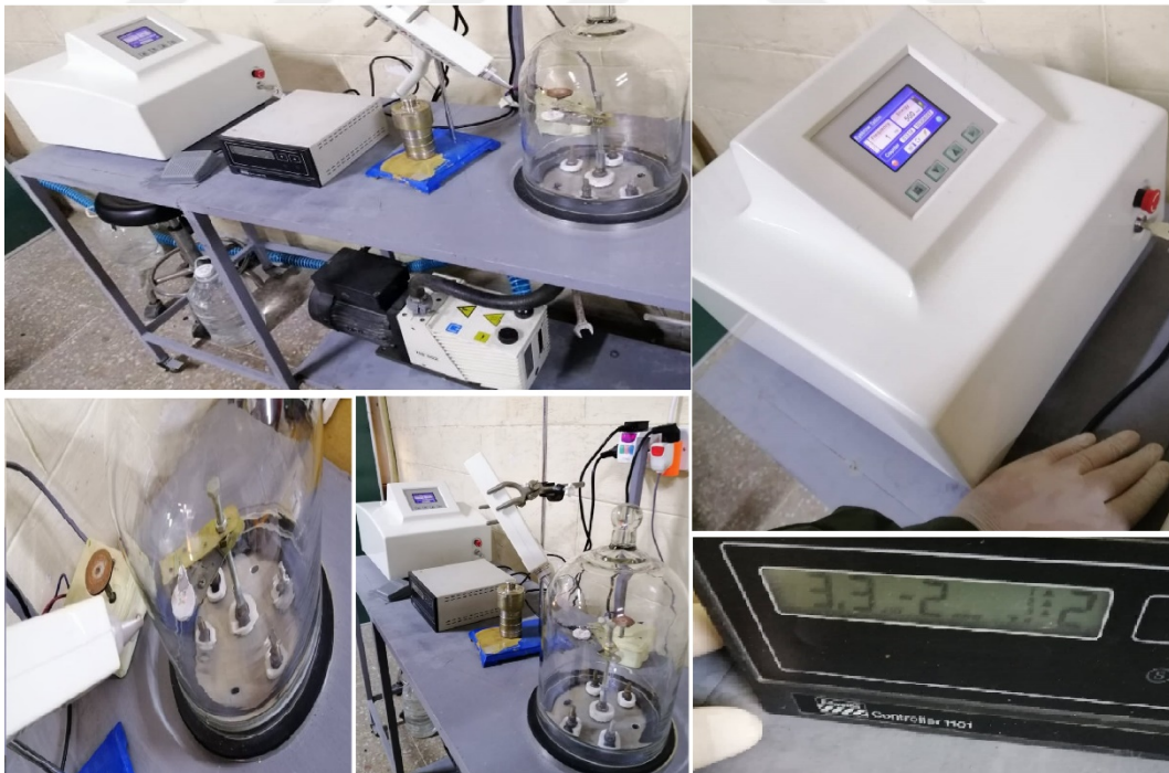
Picture 3.4. Deposition process by pulsed laser deposition technique (PLD) at the University of Baghdad.
