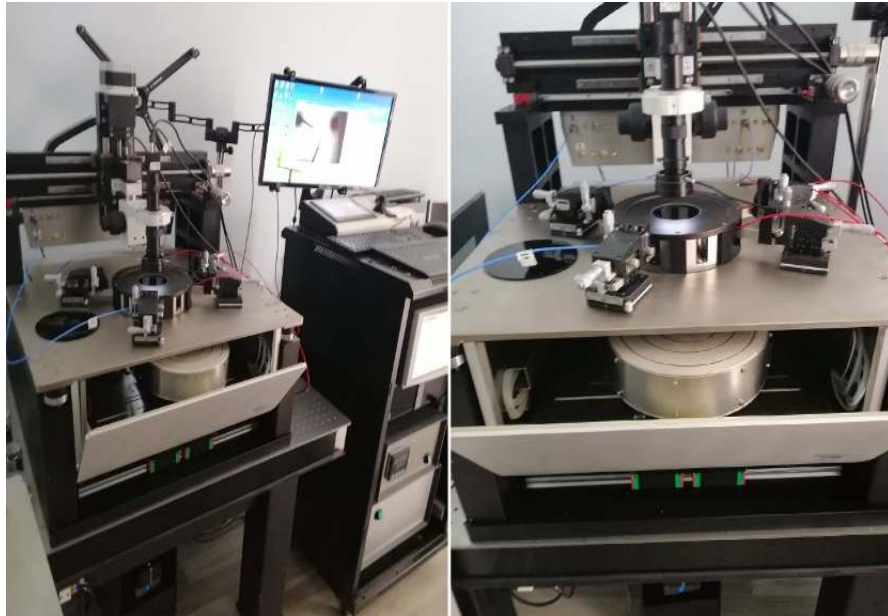
Picture 3.1. I-V measurement system at NURDAM.
