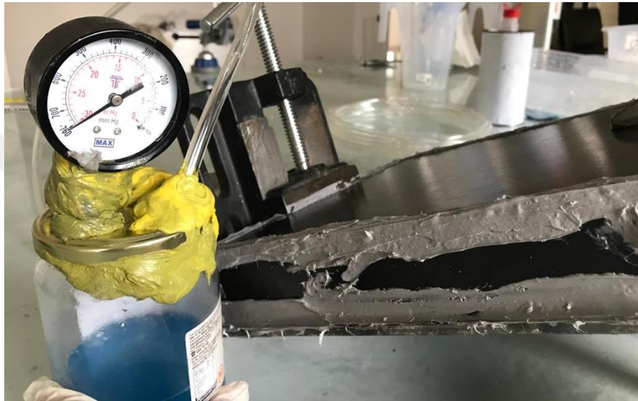
Figure 3.10. Mold under absolute vacuum
