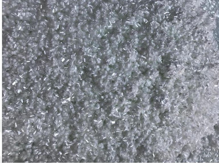
Figure 3.8. Mixture of chopped glass fibers and EPS beads
