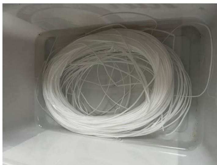
Figure 3.13. Water post-treatment of hollow fiber membranes
