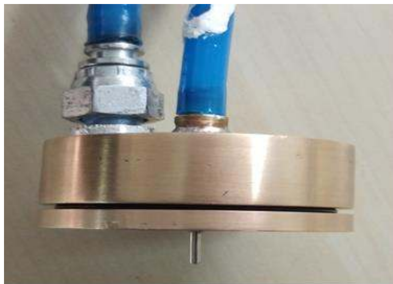
Figure 3.5. Spinneret used in hollow fiber production
