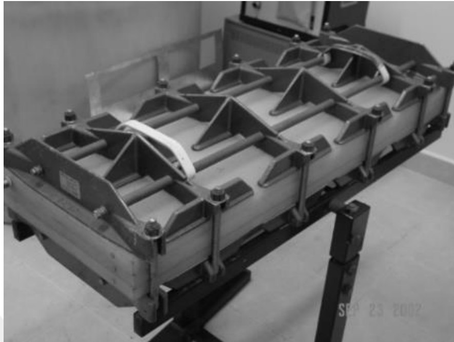
Figure 2.3. Kiil Dialyzer from 1960's [19].
