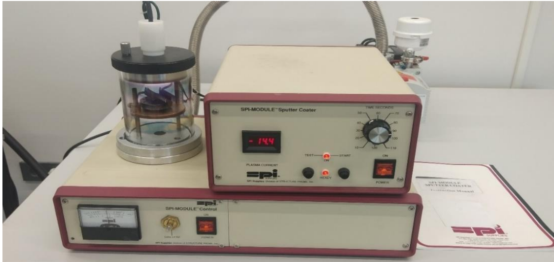
Figure 3.21. SPI gold sputter coater used to coat membrane samples for SEM analysis
