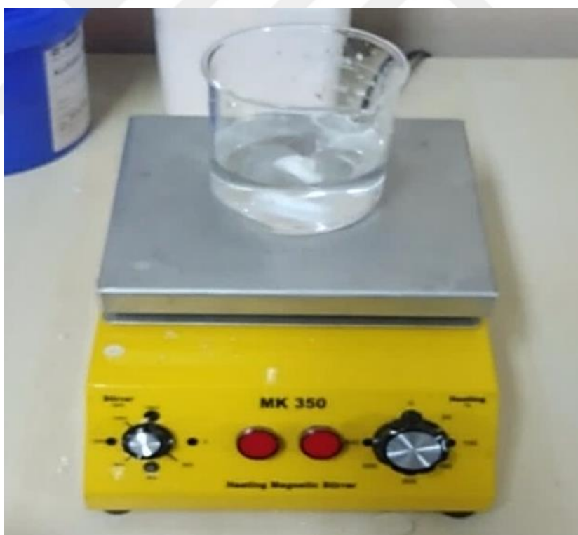
Figure 3.8. Magnetic stirrer used for producing the dope solution
