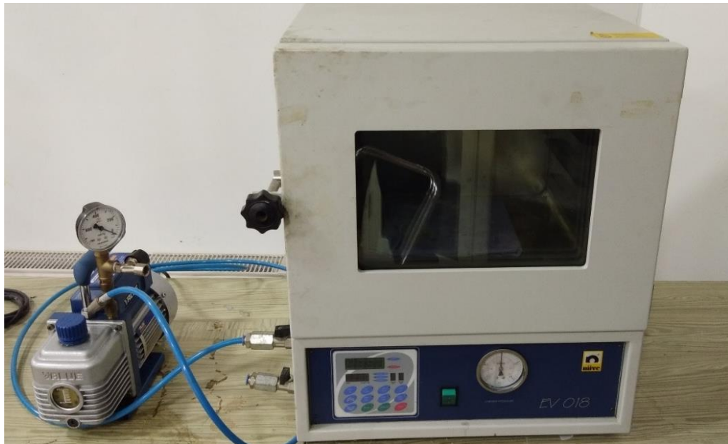
Figure 3.9. Vacuum chamber to remove residual air bubbles in the dope solution.
