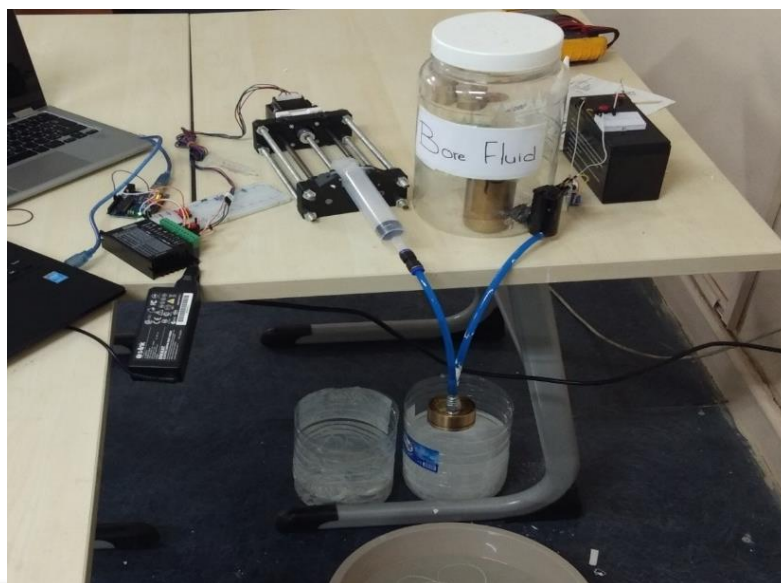
Figure 3.12. Hollow fiber spinning setup.
