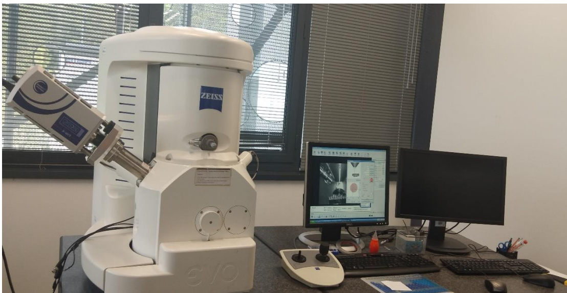
Figure 3.19. ZEISS EVO scanning electron microscope (SEM).
