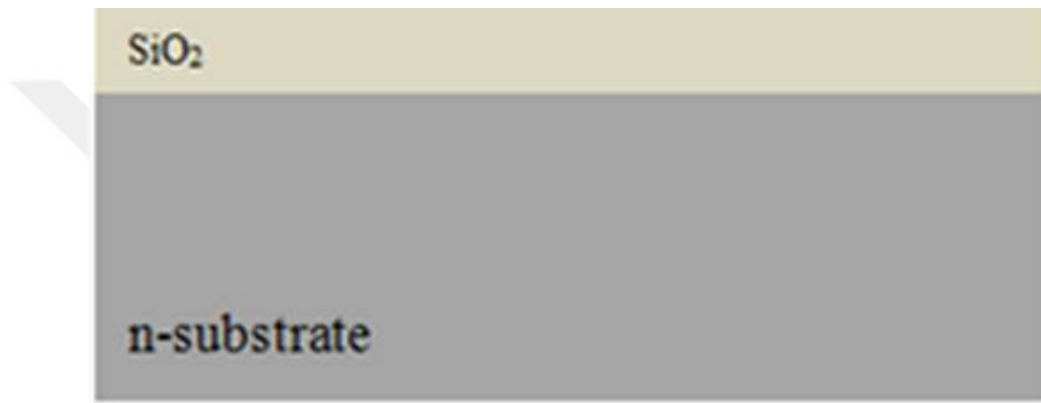
Figure 6.1. 1\text{ }\mu\text{m} \text{SiO}_2 thick grown field oxide layer on the n-type silicon substrate.
