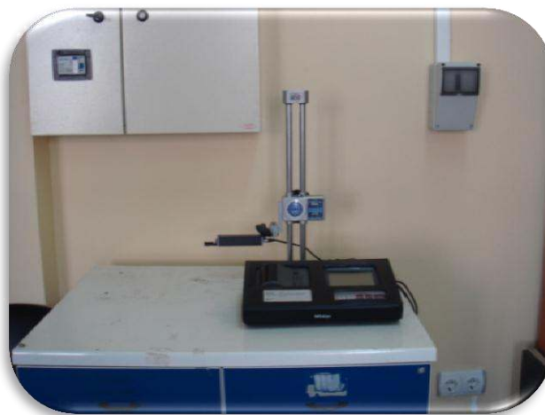
Figure 3.22 Mitutoyo SJ-301 surface (Tribology Lab., DEU)
