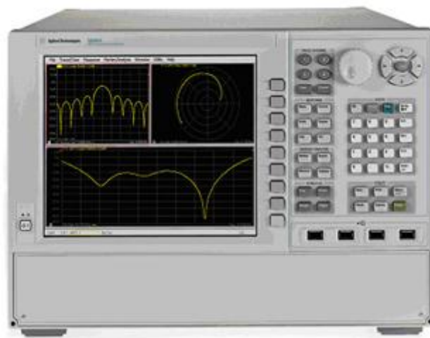
Figure 3.28 Network analyzer test machine (Electronic Material Production Lab., EMUM-DEU)
