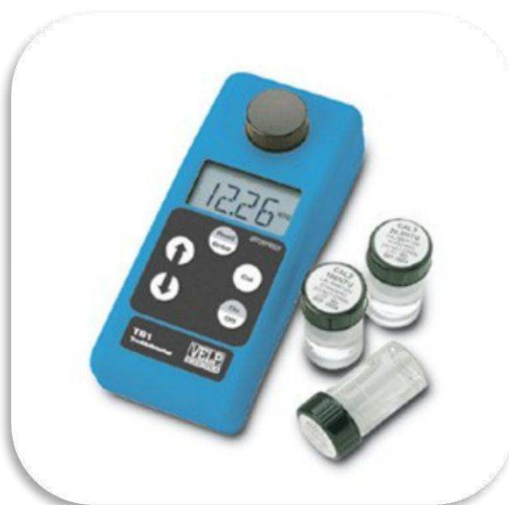
Figure 3.12 TB1 Turbid meter, VELP, Scientifics Srl, Italy (Chemistry Lab., DEU)
