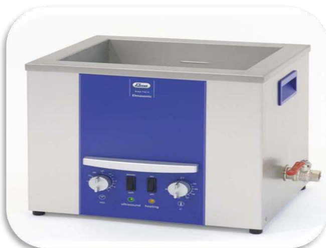
Figure 3.2 The ultrasonic bath/cleaning machine (Chemistry Lab., DEU)
