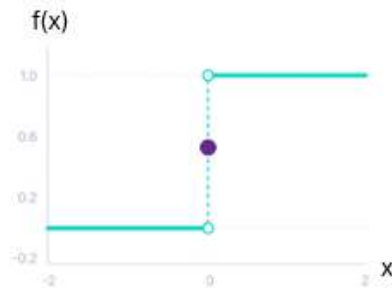
Figure 2.9 Binary Step Function [19]
