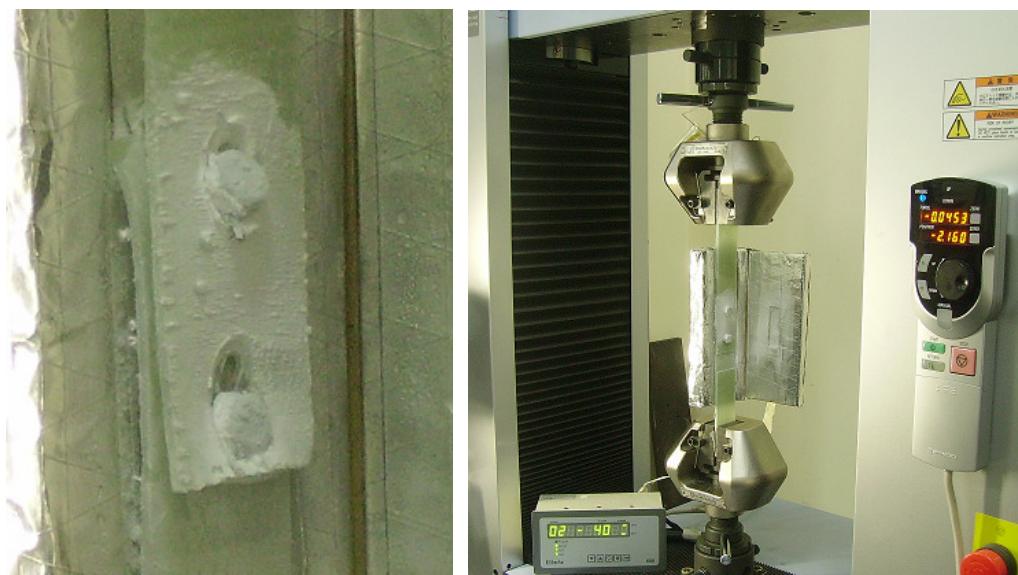
Figure 8.2 Set-up of low temperature test, thermocouple and insulation equipment
