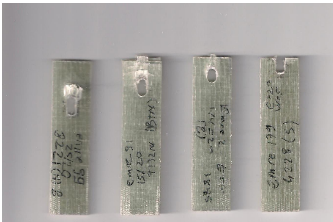
Figure 4.12 Specimens used in experiments – W= 20 mm (immersed condition)
