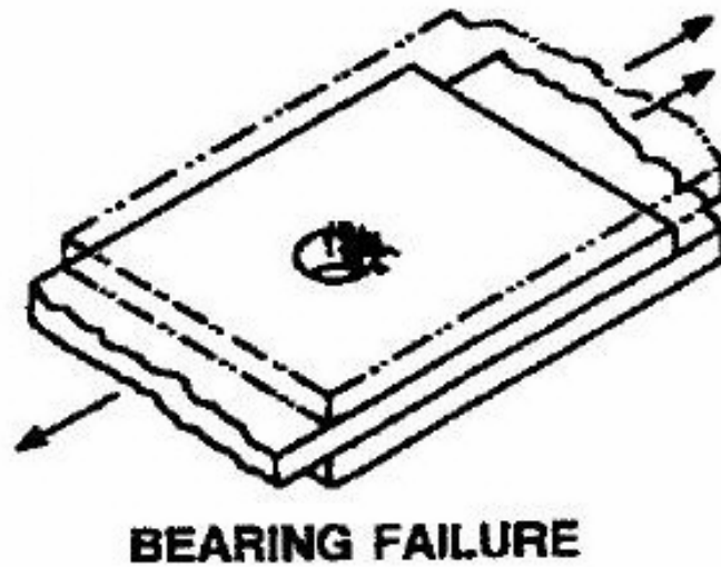
Figure 3.12 Bearing failure mode of the pinned-joint configuration (Jones, 1999)
