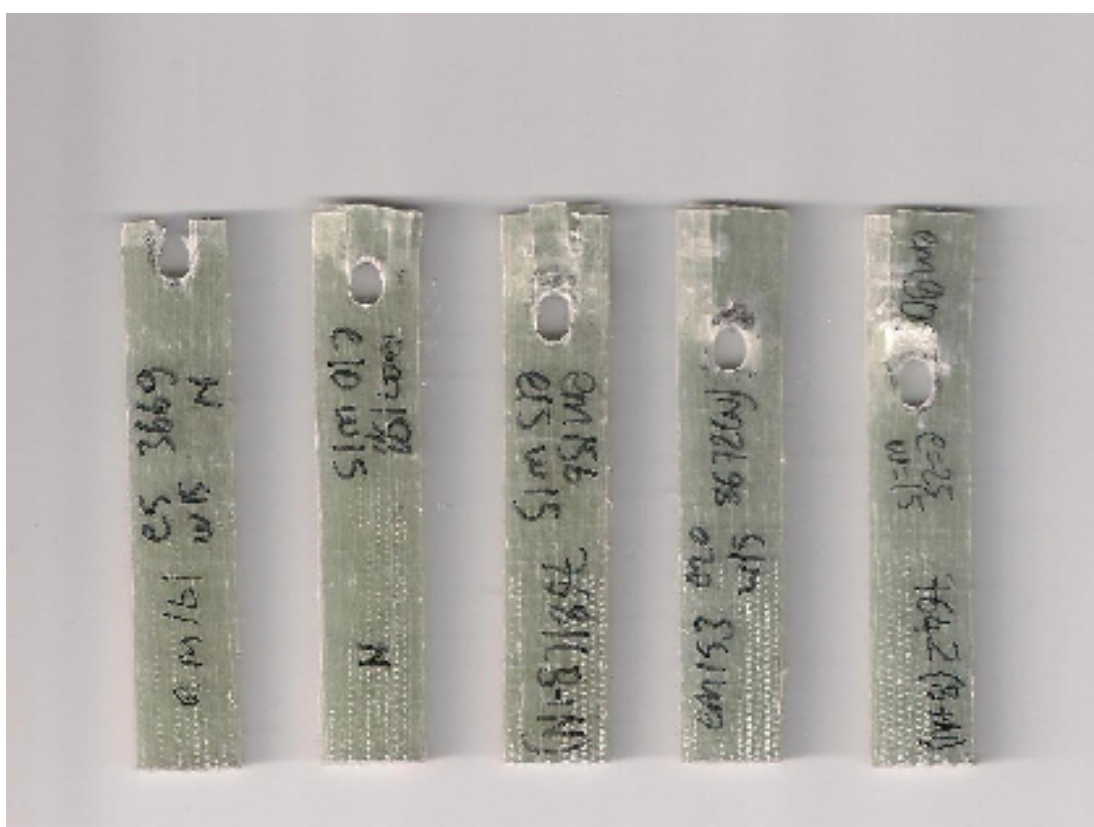
Figure 4.8 Specimens used in experiments – W= 20 mm (unimmersed condition)
