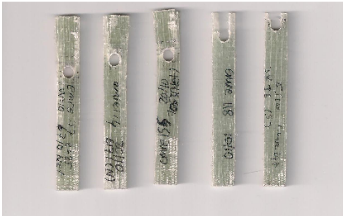
Figure 4.14 Specimens used in experiments – W= 10 mm (immersed condition)
