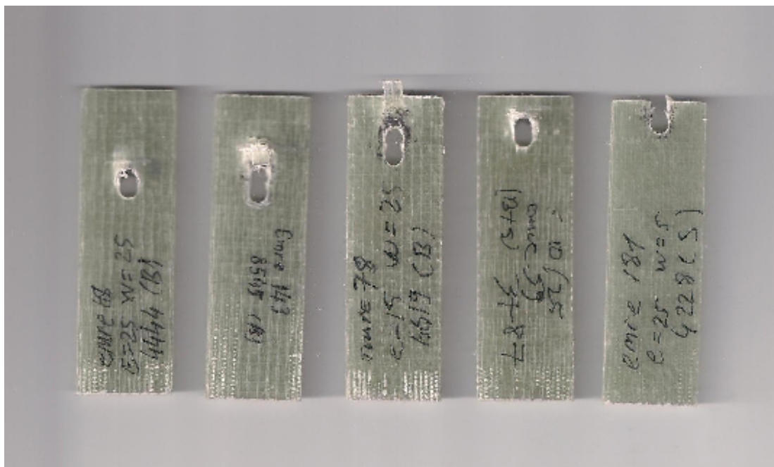
Figure 4.11 Specimens used in experiments – W= 25 mm (immersed condition)
