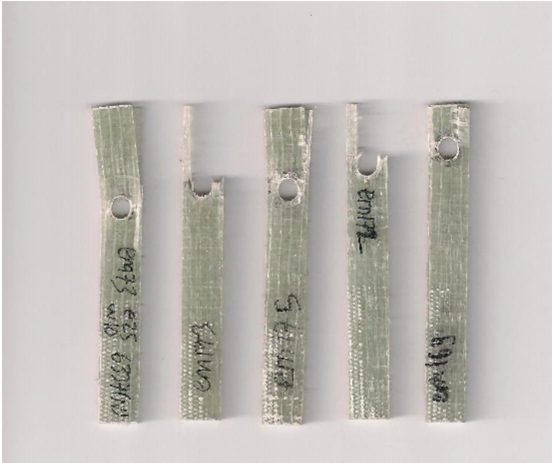
Figure 4.10 Specimens used in experiments – W= 10 mm (unimmersed condition)
