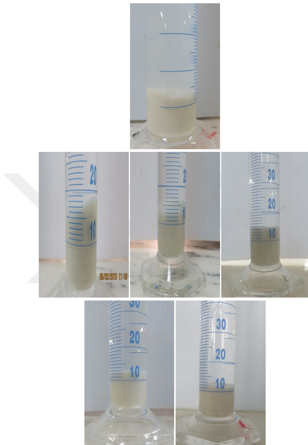
Figure A-14. Swell index of B-9 in: a) Deionized water (DIW), b) 10 mM NaCl c) 20 mM NaCl d) 30 mM NaCl, e) 5 mM \text{CaCl}_2 , f) 10 mM \text{CaCl}_2 (Personal archive, 2019)
