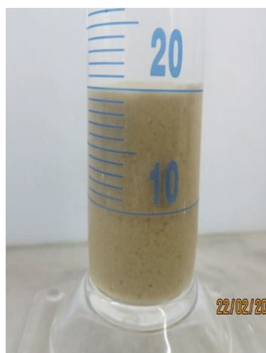
Figure A-3. Swell index of GCL-3 in: a) Deionized water (DIW), b) 10 mM NaCl, c) 20 mM NaCl d) 30 mM NaCl, e) 10 mM \text{CaCl}_2 (Personal archive, 2019)
