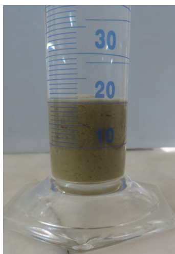
Figure A-6. Swell index of B-1 in: a) Deionized water (DIW), b) 10 mM NaCl, c) 20 mM NaCl d) 30 mM NaCl, e) 5 mM \text{CaCl}_2 , f) 10 mM \text{CaCl}_2 (Personal archive, 2019)
