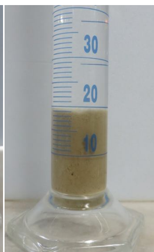
Figure A-6. Swell index of B-1 in: a) Deionized water (DIW), b) 10 mM NaCl, c) 20 mM NaCl d) 30 mM NaCl, e) 5 mM \text{CaCl}_2 , f) 10 mM \text{CaCl}_2 (Personal archive, 2019)
