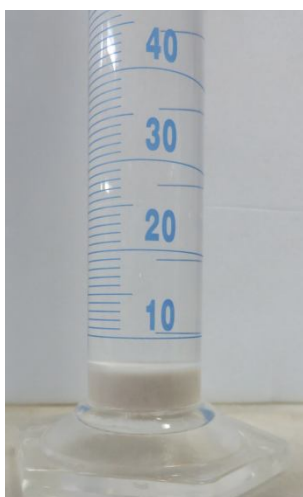
Figure A-9. Swell index of B-4 in: a) Deionized water (DIW), b) 10 mM NaCl c) 20 mM NaCl, d) 30 mM NaCl, e) 10 mM \text{CaCl}_2 (Personal archive, 2019)
