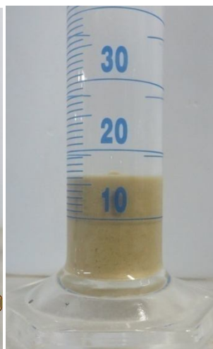
Figure A-3. Swell index of GCL-3 in: a) Deionized water (DIW), b) 10 mM NaCl, c) 20 mM NaCl d) 30 mM NaCl, e) 10 mM \text{CaCl}_2 (Personal archive, 2019)
