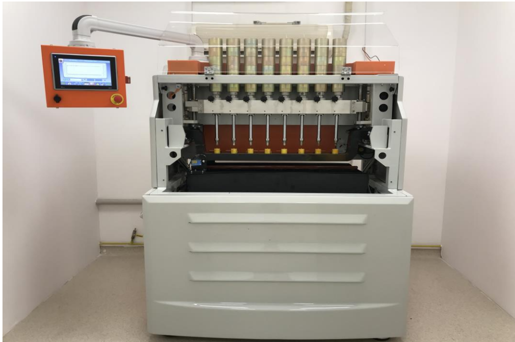
Figure 3.8. An in-vitro wear testing machine, chewing simulator Dent-Arge/ACS 8.1 (Benart, Ankara, Turkey)
