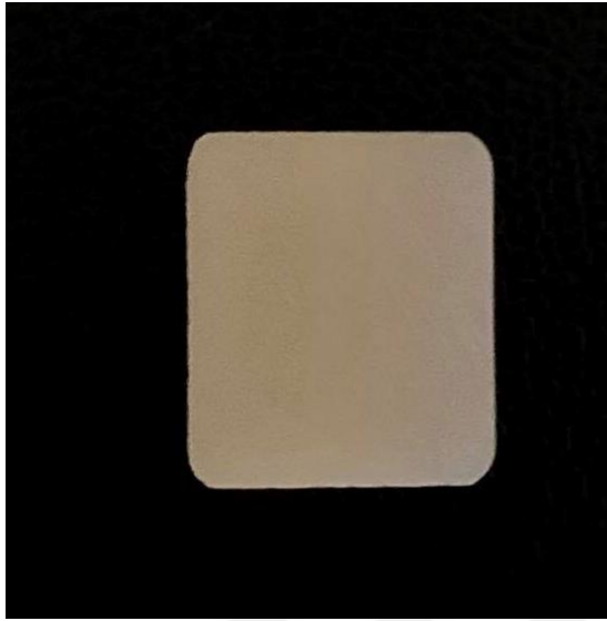
Figure 3.23: Polychromatic sample for IPS Empress CAD with shade degradation
