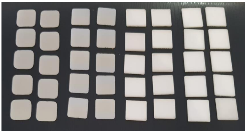
Figure 3.24: Square shaped specimens for optical tests (12 mm x 12 mm x 1.2 mm)
