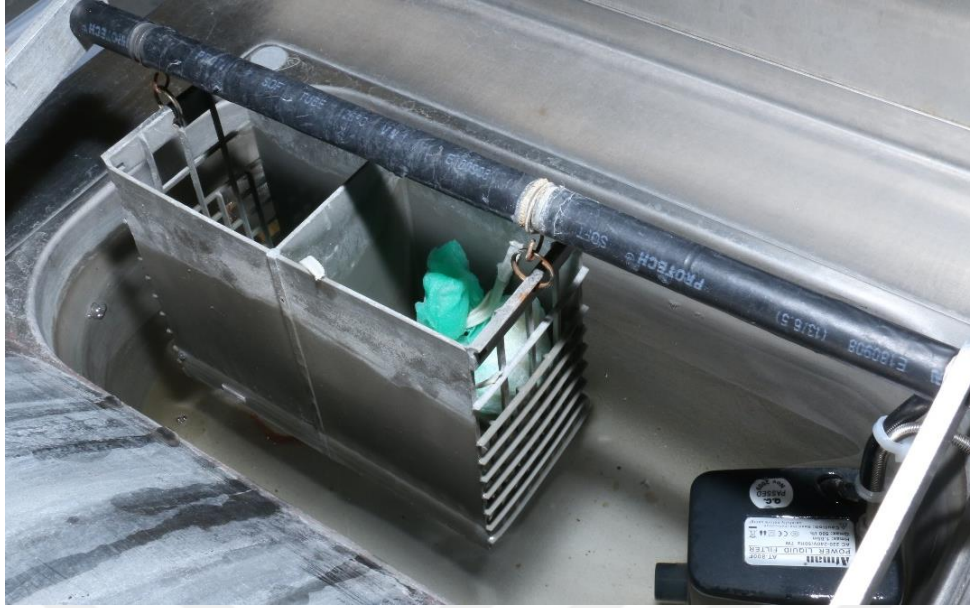
Figure 3.16: Specimens inside the bowl for thermal aging
