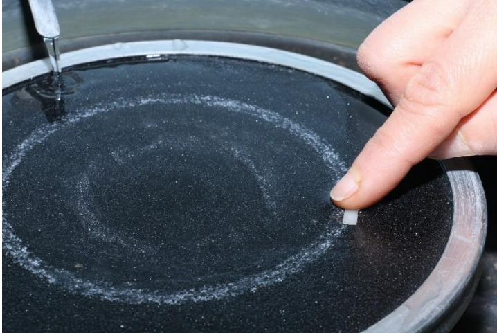
Figure 3.10: Polishing of the specimens
