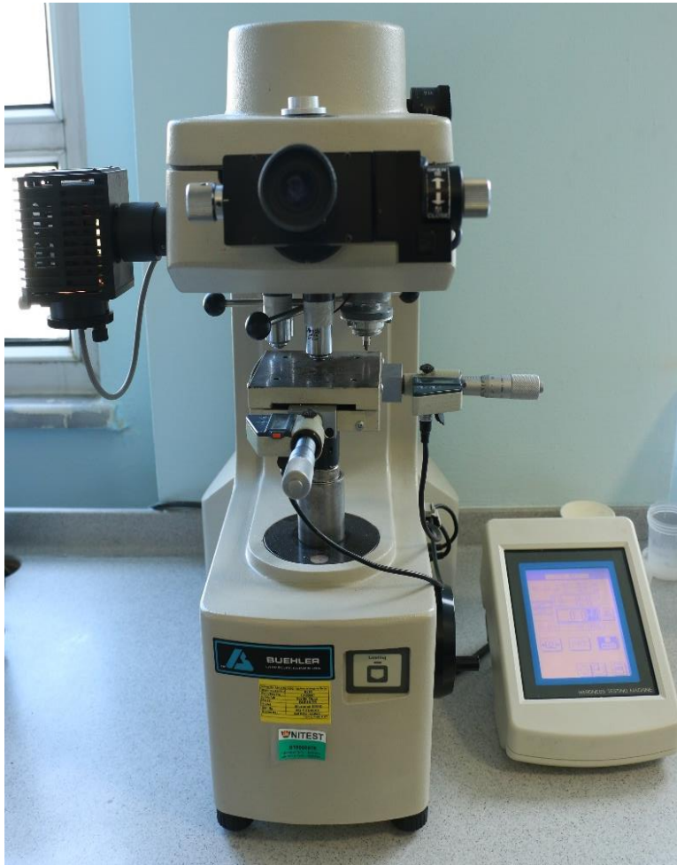
Figure 3.20: The indentation tester (Model 1600-6125, Buehler, Lake Bluff, Illinois USA)
