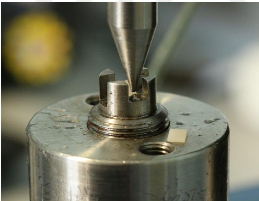
Figure 3.19: The fractural specimen at constant crosshead speed of 0.5 mm/min
