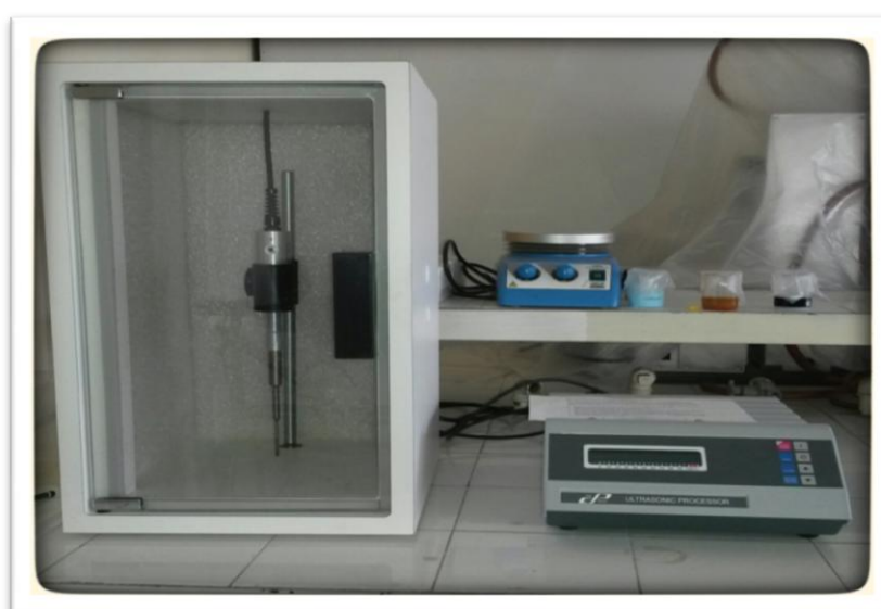
Figure 4.2 Ultrasonic generator (VCX 500, SONICS, 175 W)
