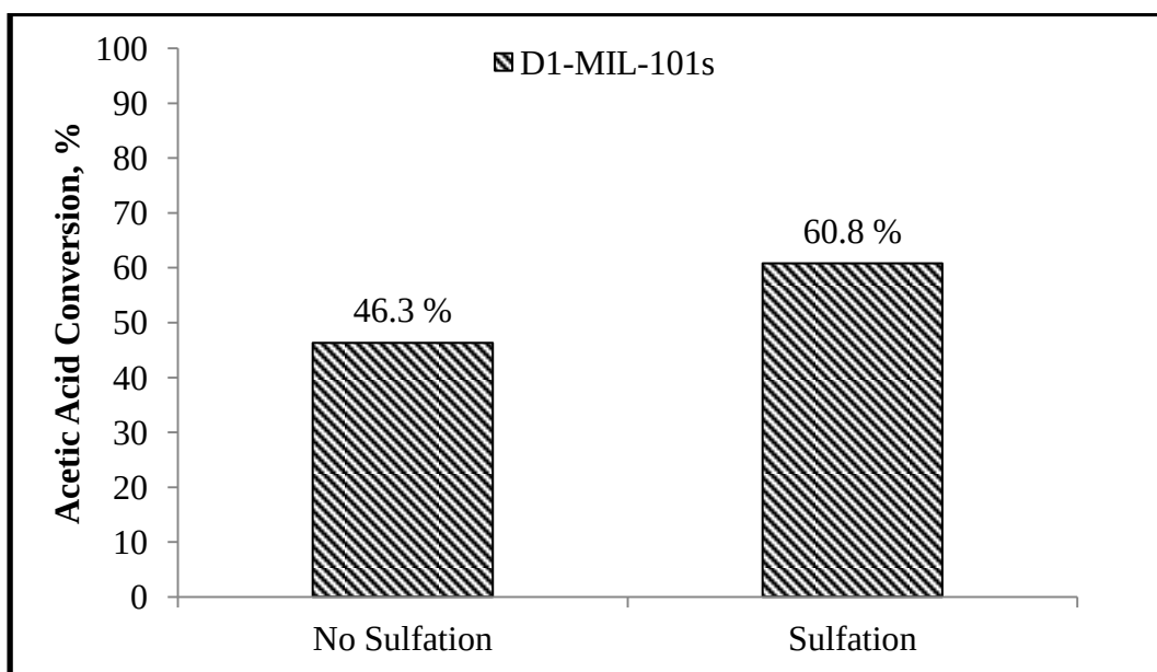
Figure 5.107 Effect of sulfation on conversion of acetic acid by using D1-MIL-101s at 363 K, 6 wt% catalysts loading, 1:1 alcohol acid ratio.
