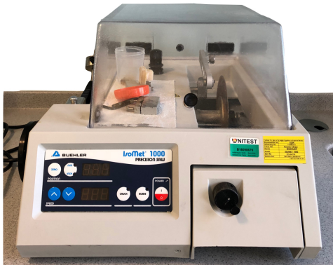
Figure 6: Precision cutting device used in the preparation of samples (Isomet 1000 (Buehler USA))
