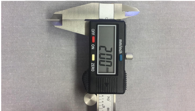
Figure 11: Measurement of sample thickness after glazing with digital caliper
