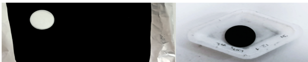
Figure 3.1. Prepared cathode film with a C/S ratio of 0.5 and sulfur loading of 1.2 \text{mg}/\text{cm}^2 .
