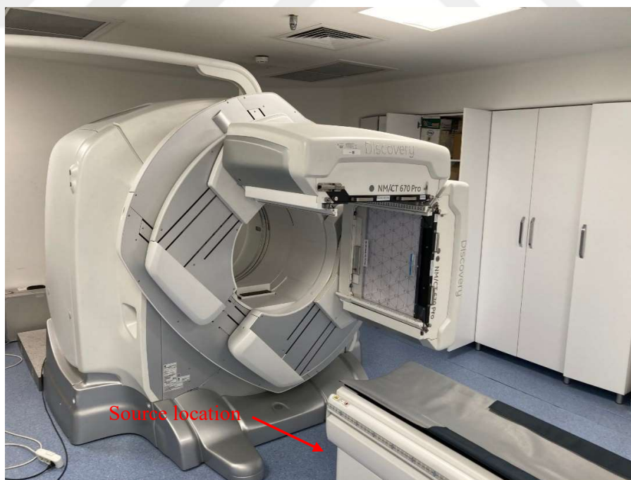
Figure 3.8. Intrinsic count rate copper plate method test setup
