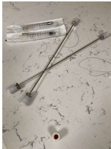
Figure 3.30. Radioactive line sources to insert water filled cylinder
