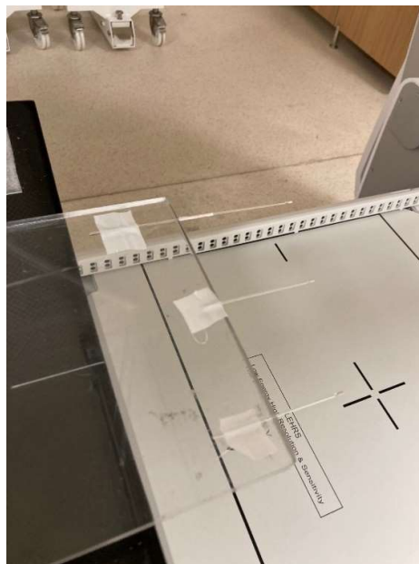
Figure 3.22. Spect reconstructed spatial resolution without scatter source positioning
