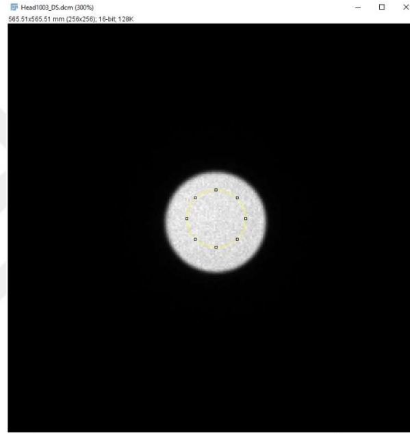
Figure 3.13. Circular ROI that is centered over the area of activity and is 60% the phantom's diameter.
