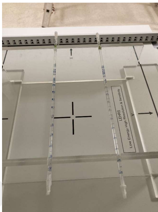
Figure 3.15. Two capillary tubes positioning parallel to collimator surface
