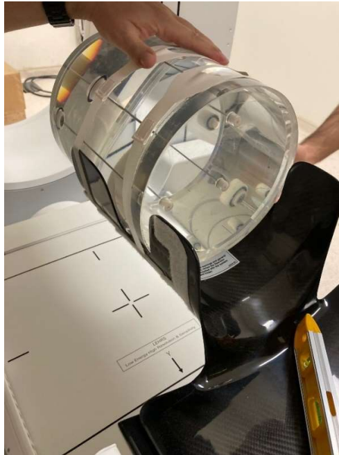
Figure 3.32. Cylinder phantom setup for system SPECT reconstructed spatial resolution test
