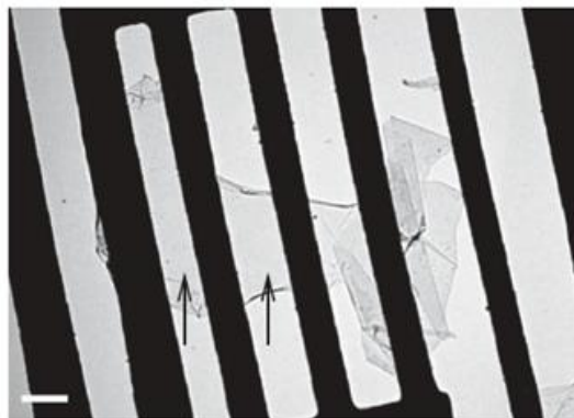
Figure 2.8 Bright-field TEM image of a suspended graphene membrane. Adapted from (Meyer et al., 2007)
