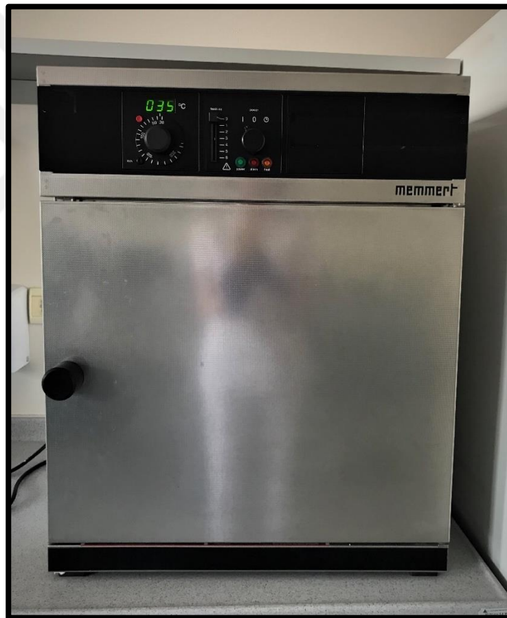
Figure 42. 37°C oven where samples were stored
