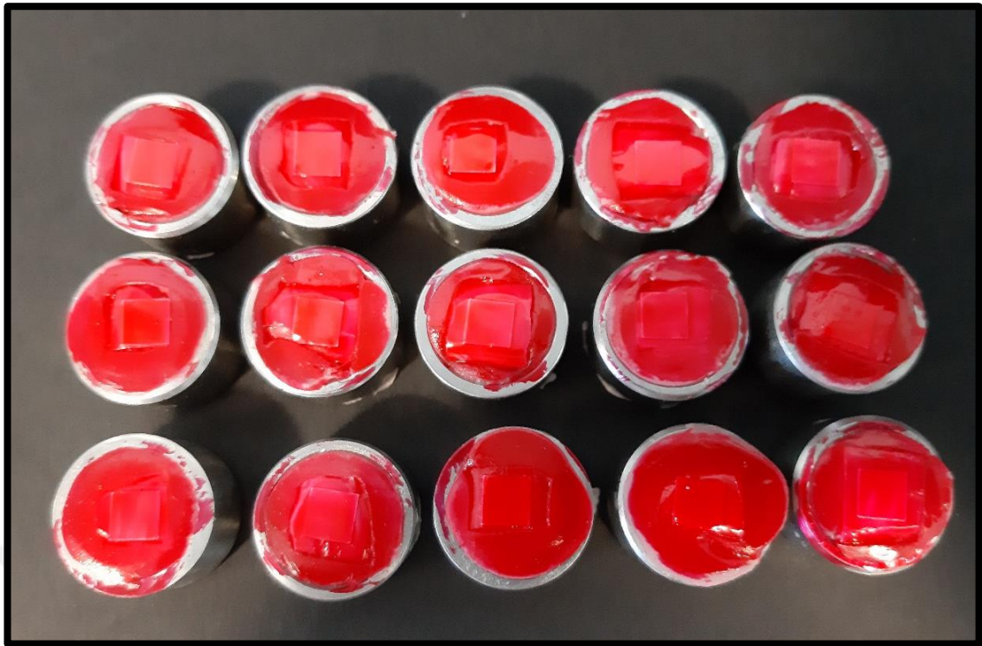
Figure 36. Polishing samples with nail polish
