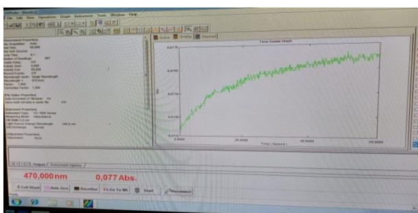
Figure 3.13. Peroxidase Enzyme Activity (POX) reading by spectrometer
