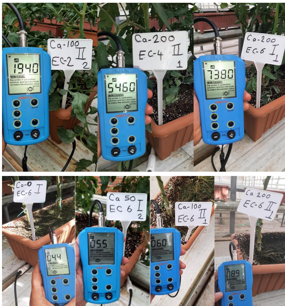
Figure 3.6. Electirictical codictivity and pH measurement in drainage solution
