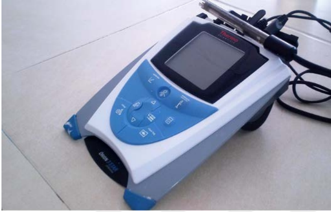
Resim 2.1. pH metre (Thermo Scientific Orion 3-Star Benchtop) (Orijinal)
