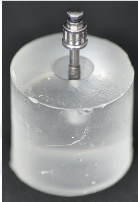
Figure 3.6. Placement of the implants in center of standardized models
