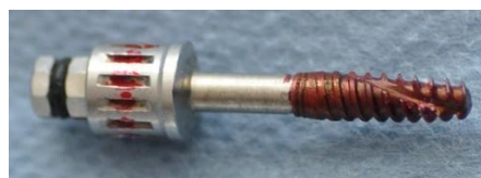
Figure 3.7. Coating implant surfaces with ink stain
