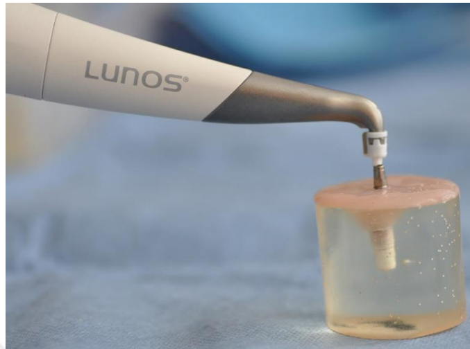
Figure 3.13. Instrumentation with the air powder abrasive device
