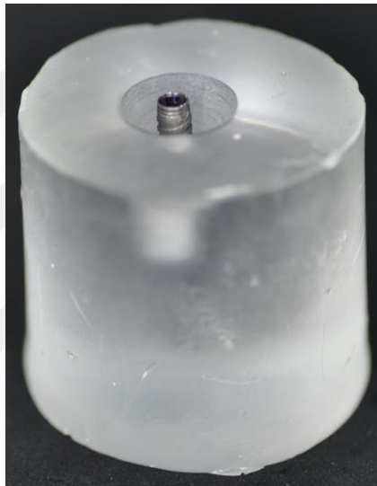
Figure 3.8. Implant margins leveled as same with the top plane of resin models
