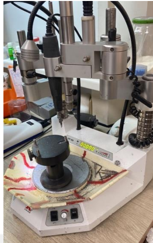
Figure 3.2. The parallellometer device with milling machine
