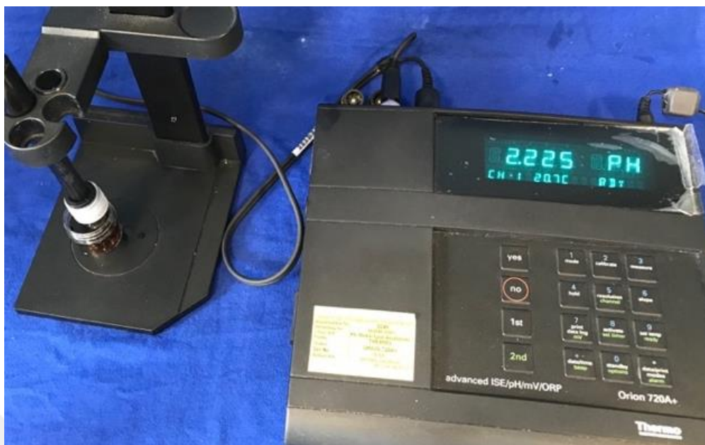
Figure 3. 11. pH measurement for Cola ( \text{pH} = 2.225 \pm 0.05 )
