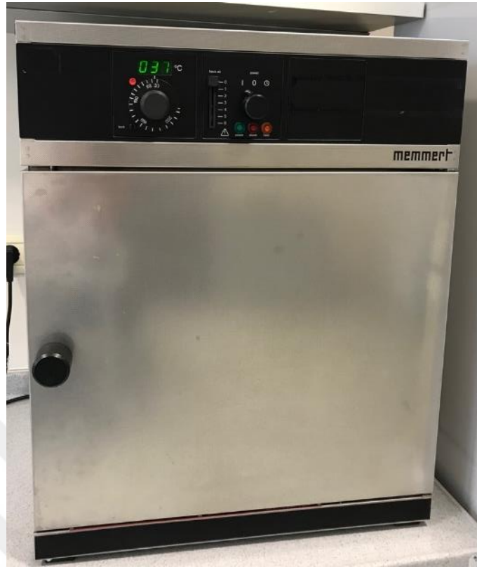
Figure 3. 15. Incubator used to control environmental conditions of immersed samples
