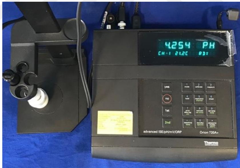
Figure 3. 10. pH measurement for Kefir ( \text{pH} = 4.254 \pm 0.05 )
