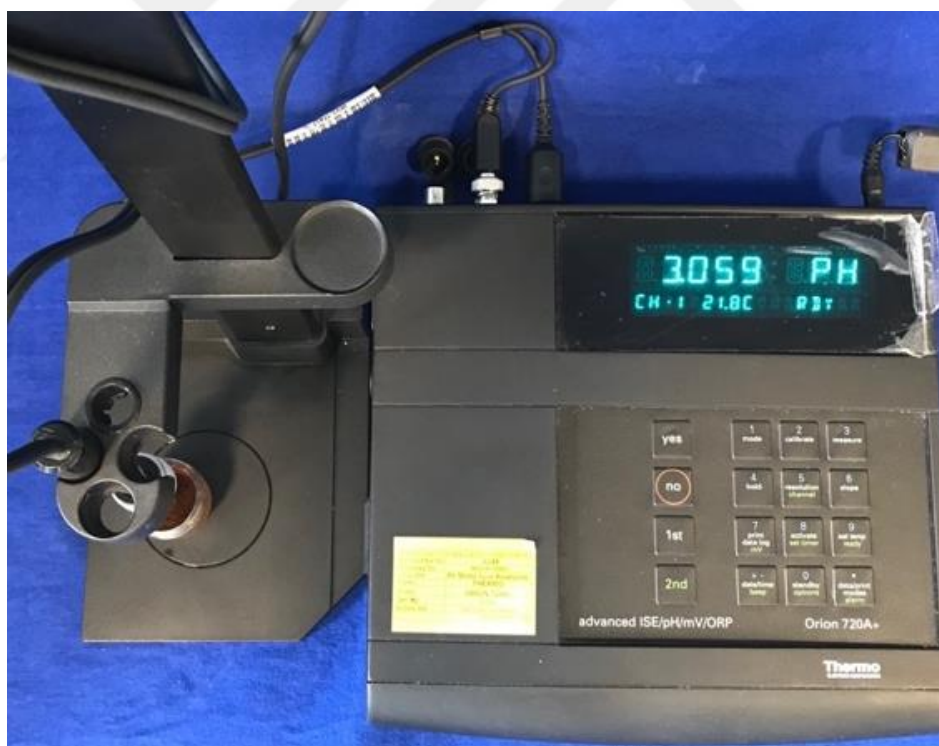
Figure 3. 12. pH measurement for iced tea ( \text{pH} = 3.059 \pm 0.05 )
