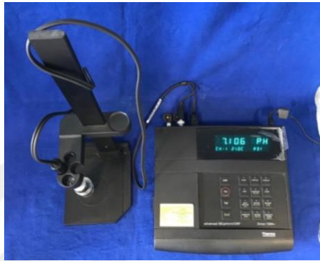
Figure 3. 3. pH level measurement of the artificial saliva by Thermo Scientific Orion 720A+ and 920A+ pH meter (Hard Tissue Laboratory; Faculty of Dentistry - University of Yeditepe)
