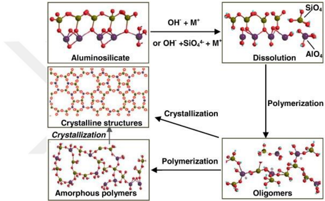
Şekil 1.2. Geopolimerleşme Modeli (Zhang, Zhu, Zhou, & Wang, 2016)
