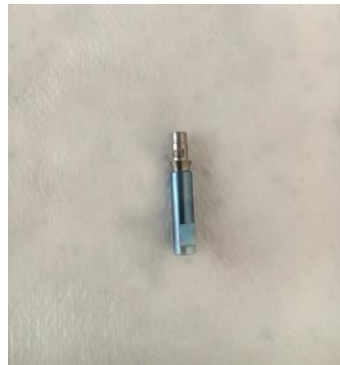
Şekil 3.1. Ti-base dental implant abutment (Grade 5) ve analogu (Bilimplant, Turkey)
