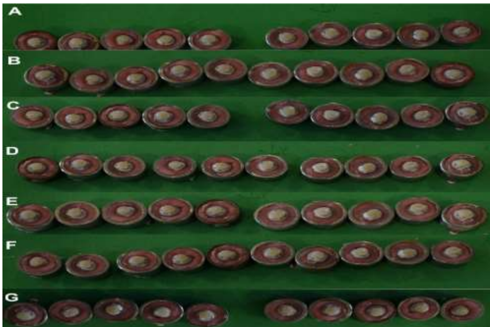
Figure 3.27. Ceramil , A.Control , B.HF Acid , C. Air blasting, D. Airblasting +Z prim Plus , E. Cojet , F .Siljet , G. Fiber Laser
