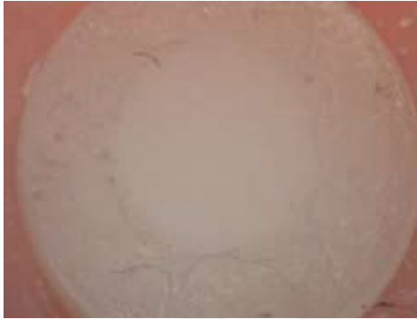
Figure 4.4. Stereomicroscope images of adhesive failure
