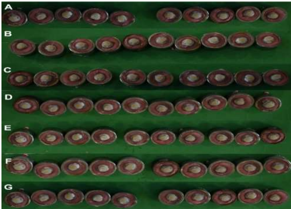
Figure 3.26. Zenostar . A ControL, B. HF Acid, C. Air Blasting, D. Air blasting+ Z prim Plus , E.Cojet , F .Siljet ,G. Fiber Laser
