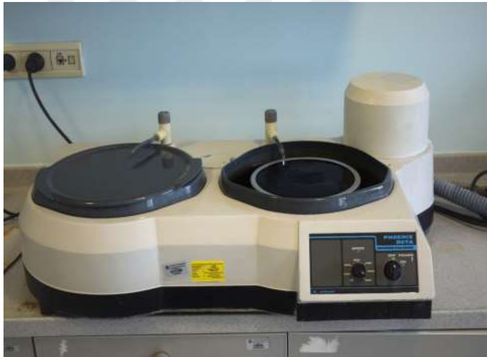
Figure 3.7. Polishing machine (Phoenix Beta Grinder/ Polisher)
