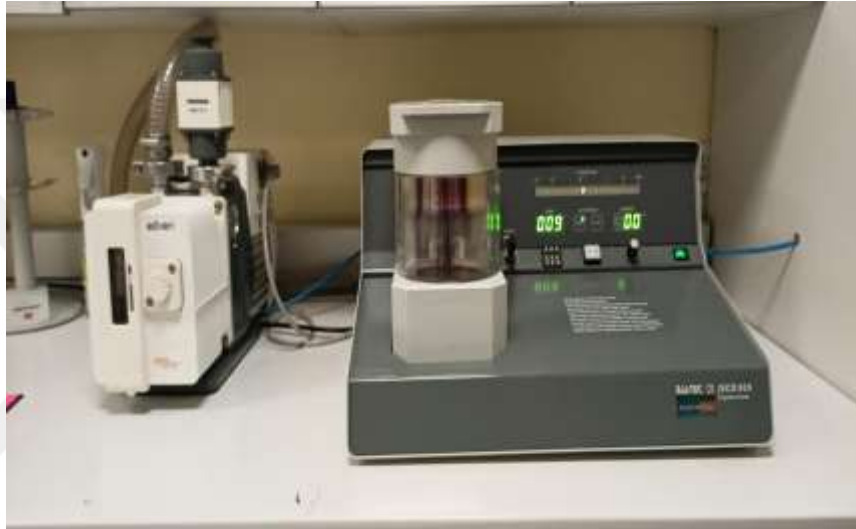
Figure 3.29. BAL-TEC (Sputter Coater SEM Sample Prep)
