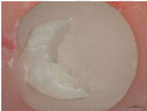
Figure 4.5. Stereomicroscope images of mixed failure
