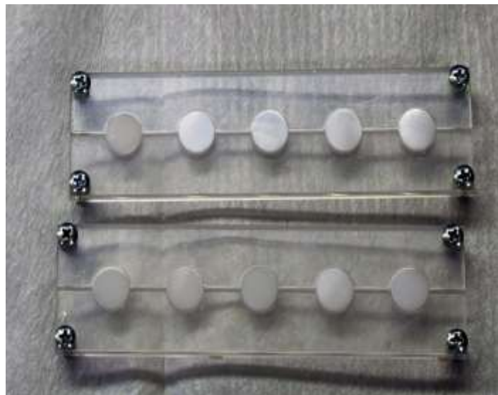
Figure 3.9. Epoxy glass mold
