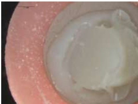
Figure 4.6. Stereomicroscope images of cohesive failure
