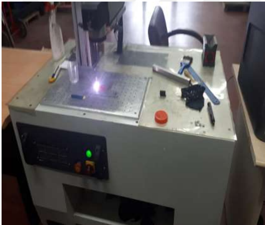
Figure 3.20. Fiber optic laser machine (Rofin-Sinar Laser GmbH Germany)
