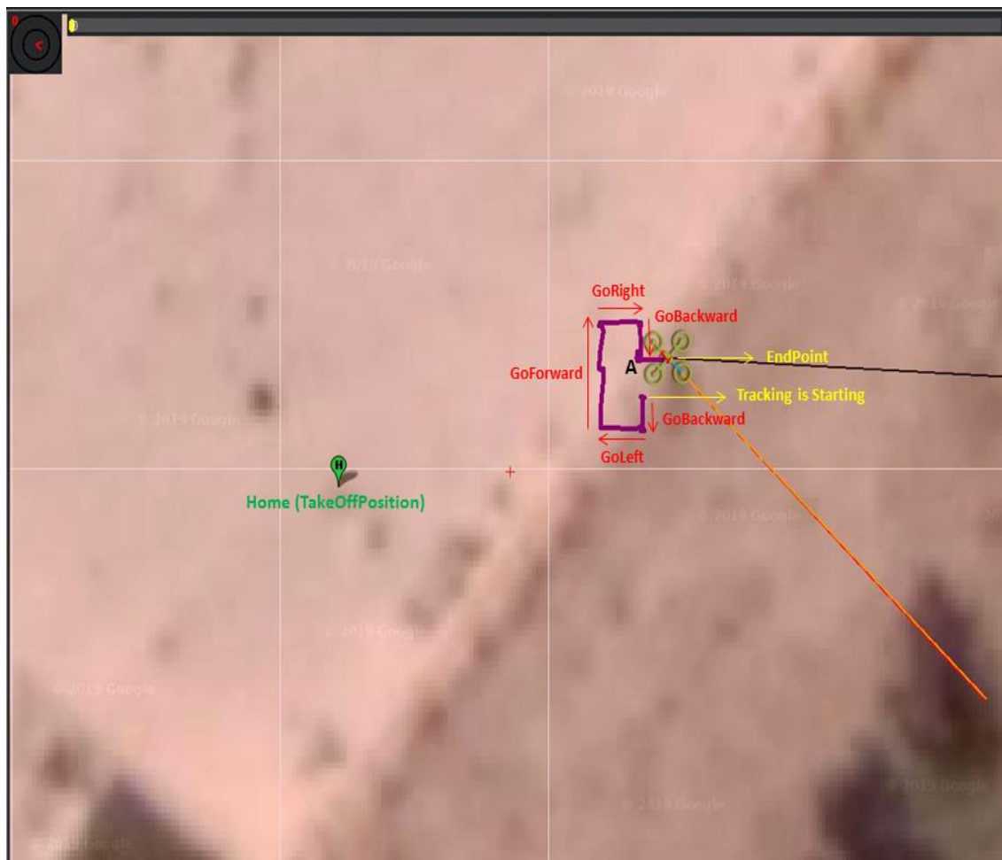
Figure 38: Illustration of 3D tracking mission
