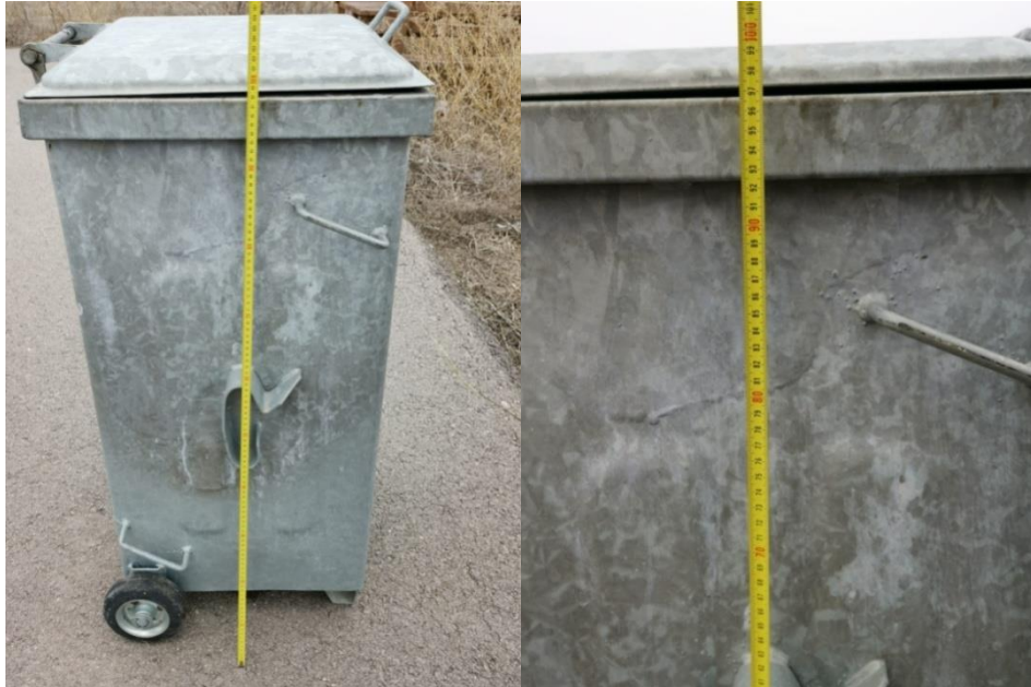
Figure 37: Measurement of displacement in z-axis (height)
