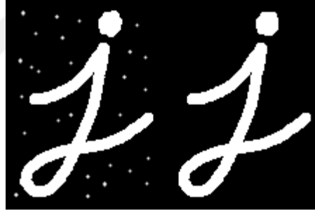
Figure 19: Result of erosion and dilation processes for removing noises [56]
