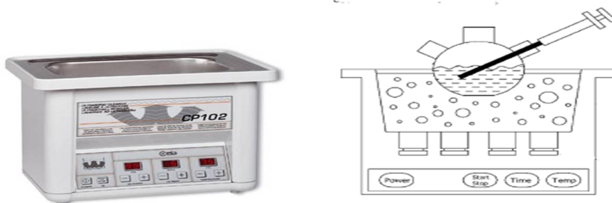
Figure 2.2. Experimental Set-up of ultrasonic bath
