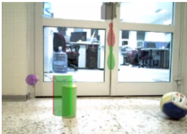
Figure 1.1: A sample object recognition output from the LINE-MOD algorithm.
