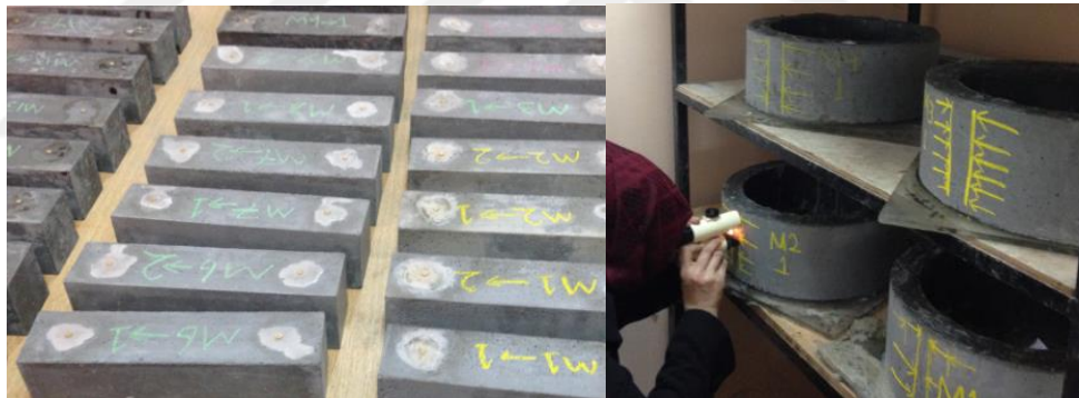
(b) Dry curing samples for dry shrinkage and restrain shrinkage
