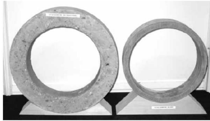
Figure 2.8. Reduction in pipe wall thickness of UHPC (right) compared to an equivalent pipe in normal concrete (left) [99]
