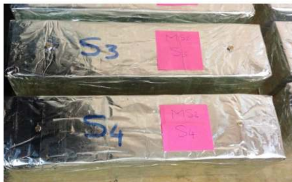
(c) Sealed curing for autogenous shrinkage
