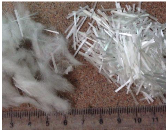
Figure 4.6. Capillary micro glass fiber within UHPC before and after addition
