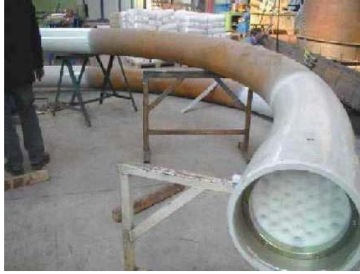
Figure 2.20. Curved saddles for stay cables in Sungai Muar Bridge [105]
