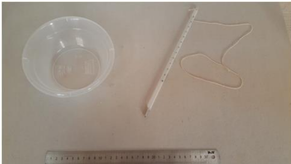
Figure 3.14 Crumb test apparatus
