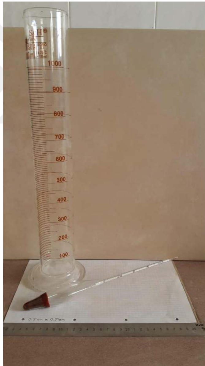
Figure 3.16 Double hydrometer test apparatus
