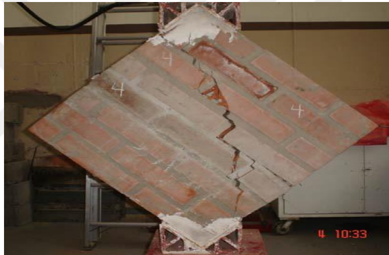
Figure 2.13. Diagonal compression test for a wall sample [24]
