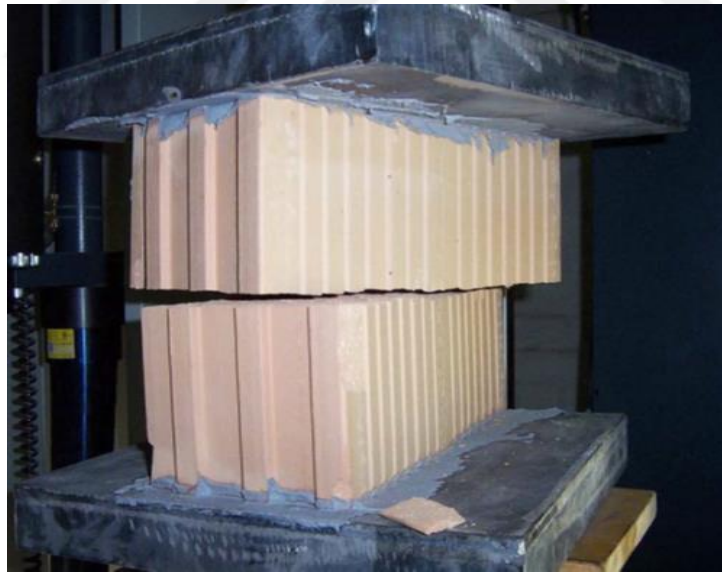
Figure 2.10. Tensile bond test for brick-mortar transition point [18]
