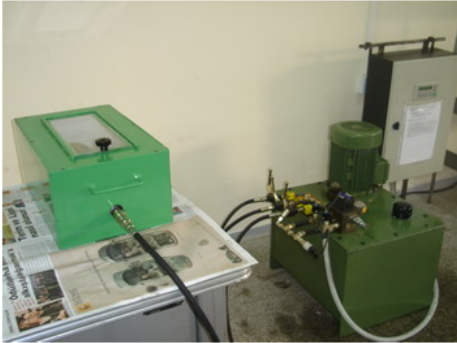
Figure 6.6 A PLC controlled servo-hydraulic testing machine.
