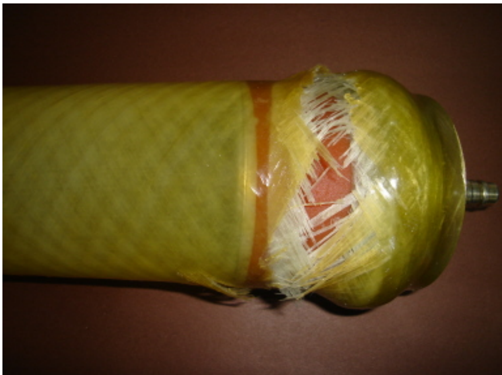
Figure 7.11 Fiber breakage damage mechanism.
