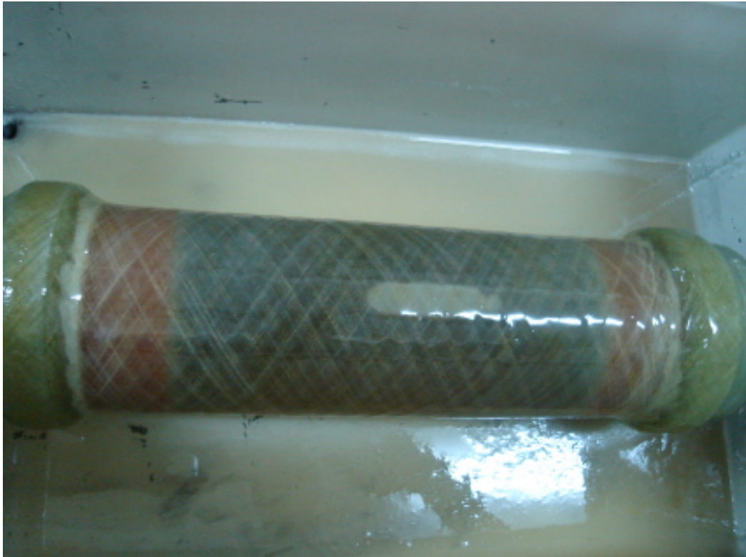
Figure 7.8 The beginning of the whitening damage mechanism.
