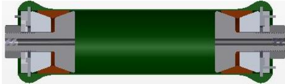
Figure 6.3 Closed-end internal pressure test apparatus.
