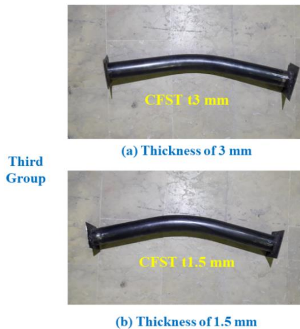
Figure 4.3 Patterns of the failures in the concrete beams (third group)
