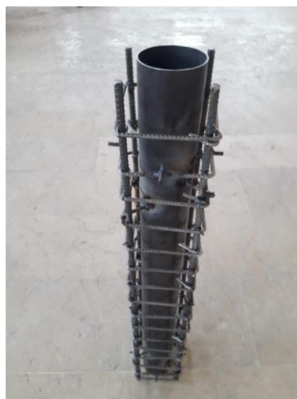
Figure 3.7 The inner part of the specimen
