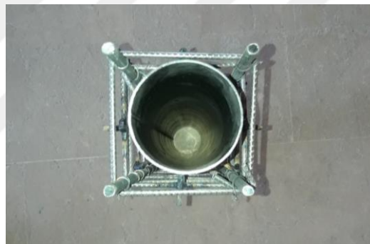
Figure 3.6 The specimen before casting (top view)
