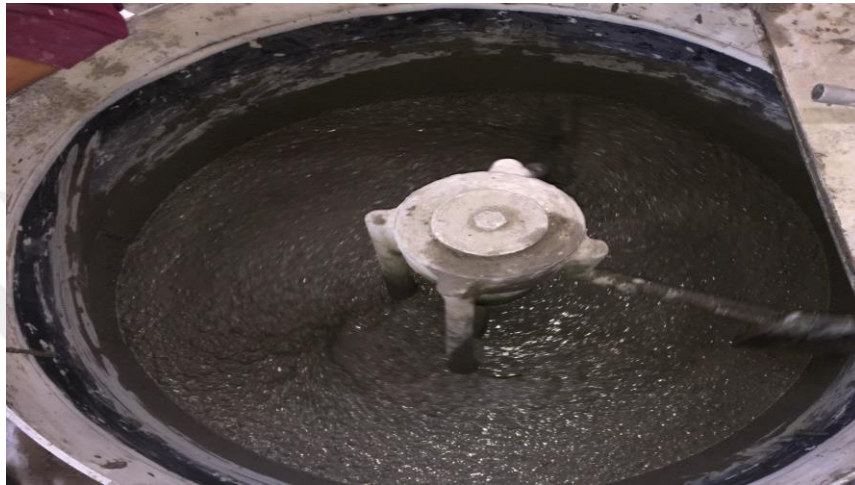
Figure 3.1 Mixing of the SCC
