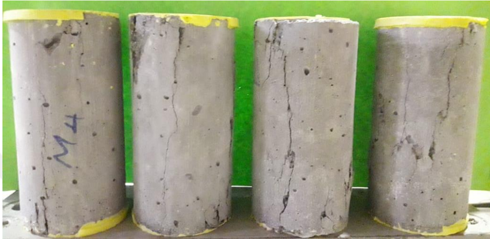
Figure 3.2 Concrete cylinders after testing
