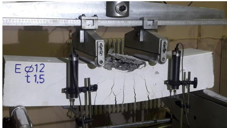
Figure 3.11 The specimen after loading
