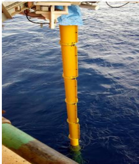
Figure 1.7. An application of faring on the pipeline ( http://i.imgur.com/AcKilqY.jpg ).
