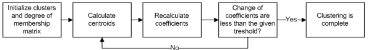
Figure 3.21. Block diagram of c-means clustering method
