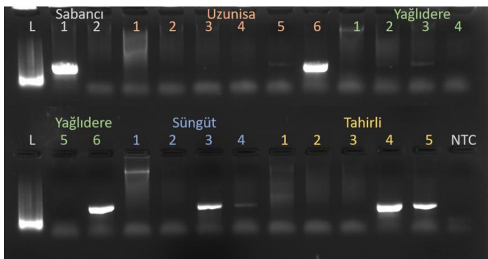
Figure 37: Gel result of the 2019 season leaf samples tested with Ec_F1-R3 primers.
