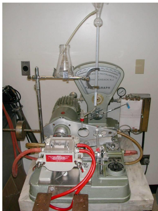
Figure 3.6 : Farinograph used for flour water absorption properties.
