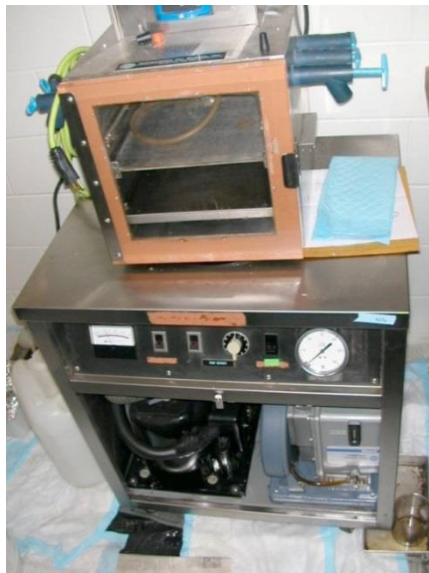
Figure 3.3 : Freeze-dryer used for bread crumb, crust and dough samples.
