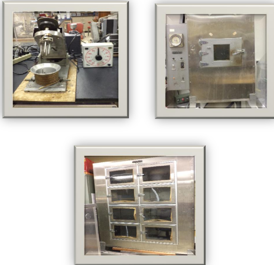
Figure 3.2 : Fermentation cabinet, rotary type oven and pin type mixer used for breadmaking.
