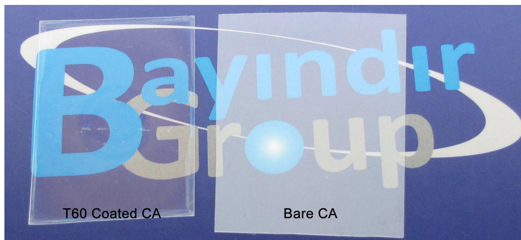
Figure 5.10: Photographs of hybrid ormosil coated and bare CA substrates visualizing antireflective property of coatings.
