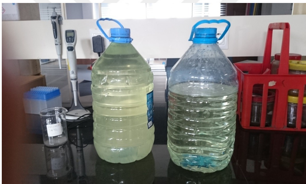
Figure 4.7. Wastewater sample taken from equilibration tank (left), filtrate obtained by the microfiltration of the wastewater using tubular ceramic MF membrane
