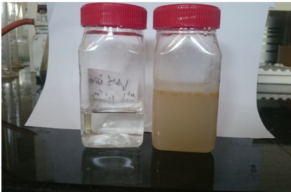
Figure 4.22. Permeate sample collected during microfiltration where the cross flow velocity and TMP were 0.16 m/s and 2 bars and oily-wastewater.
