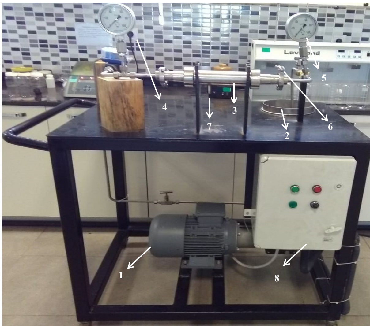
Figure 3.4. Filtration equipment used in this thesis 1. Feed pump, 2. Feed tank, 3. Membrane module, 4. Pressure gauge (membrane inlet), 5. Pressure gauge (membrane outlet), 6. Needle valve, 7. Permeate outlet, 8. Pump controller
