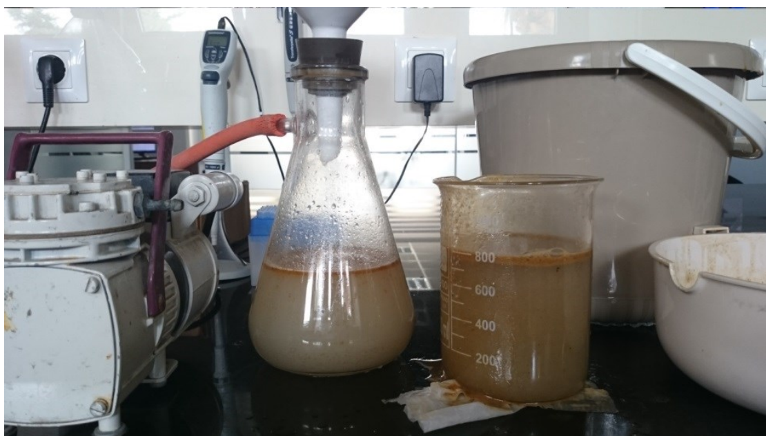
Figure 4.3. Wastewater obtained before oil removal by fat-trap system before (right) and after (left) filtration through general purpose filter paper
