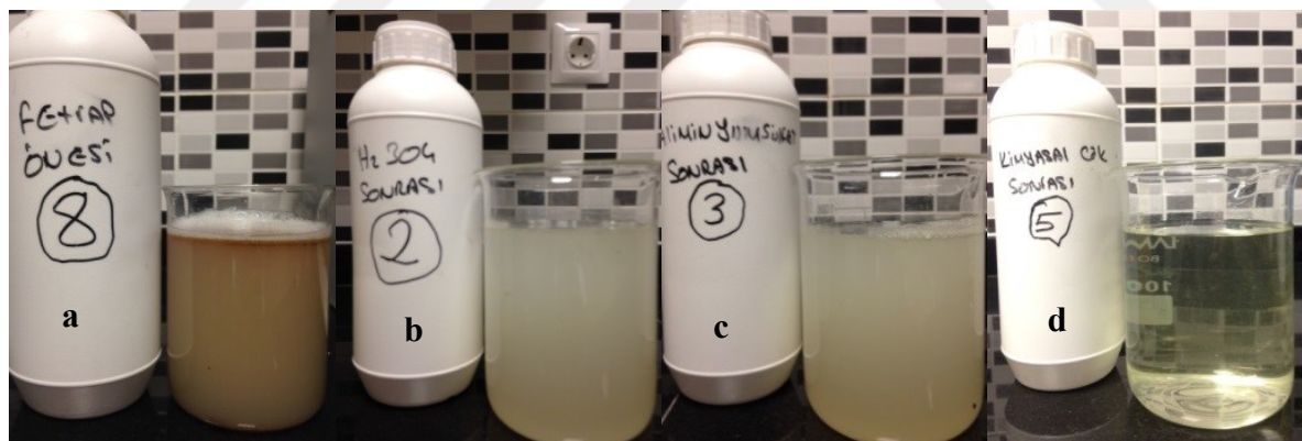
Figure 4.2. Wastewaters a. before fat trap, b. after \text{H}_2\text{SO}_4 addition, c. after \text{Al}_2(\text{SO}_4)_3 addition, and d. from equilibration.
