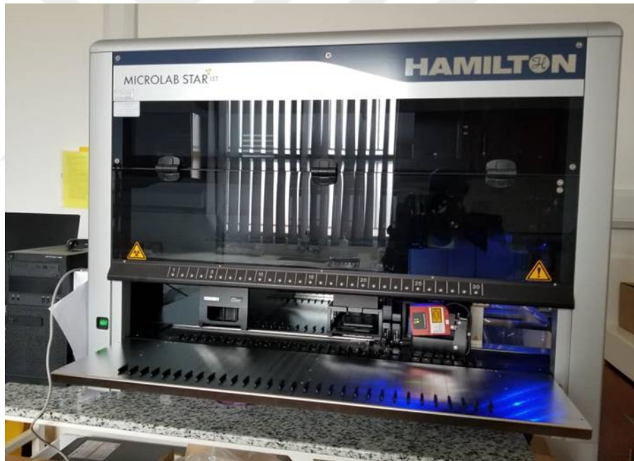
Figure 4 Hamilton Bio-robots used for Extraction.
