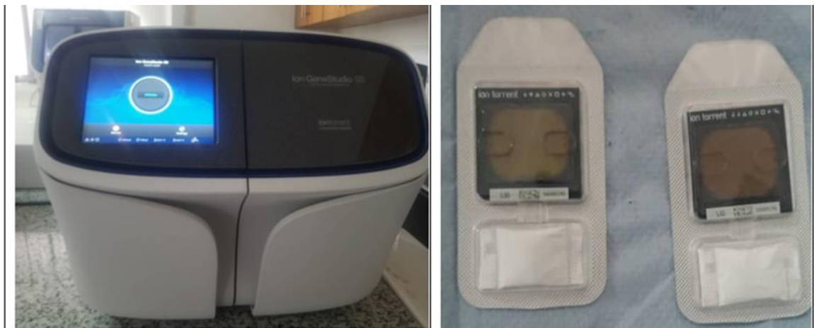
Figure 7. The Gene Studio and the 530 Chips used for Sequencing of the samples.
