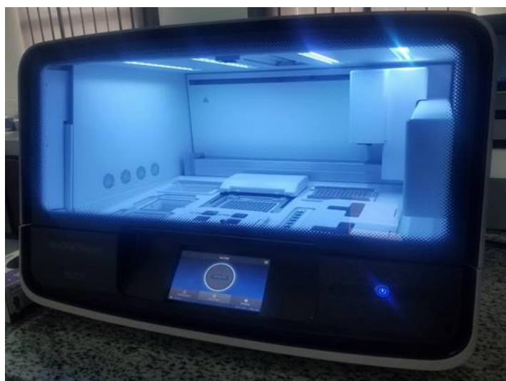
Figure 6 The Ion Chef Instrument used for Library and Template preparations.
