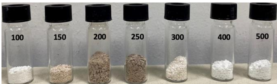
Figure 3.1: Color differences on \text{TiO}_2 samples after calcination. (250 mg of Degussa P25 and 3 mL of ethanol were mixed for all samples, calcination temperatures (in ^{\circ}\text{C} ) were labeled on the vials).
